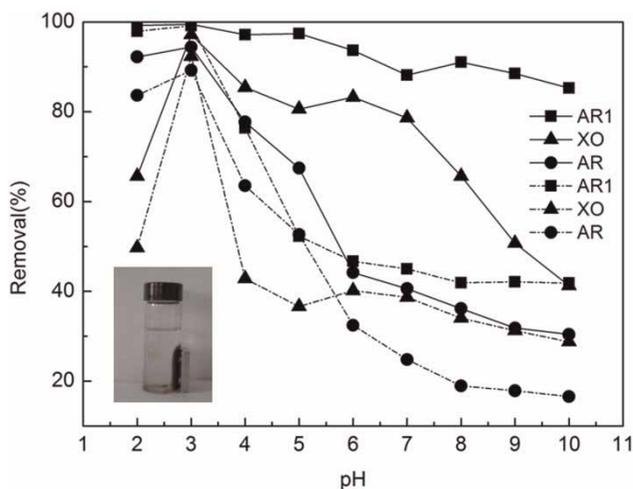
Figure 2 | Effect of pH on adsorption (solid line and dashed line represent CS/EPTAC/Fe<sub>3</sub>O<sub>4</sub> and CS/Fe<sub>3</sub>O<sub>4</sub>, respectively).
