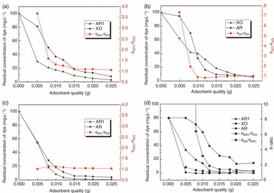
**Figure 5** | Competitive adsorption in the multicomponent systems.
