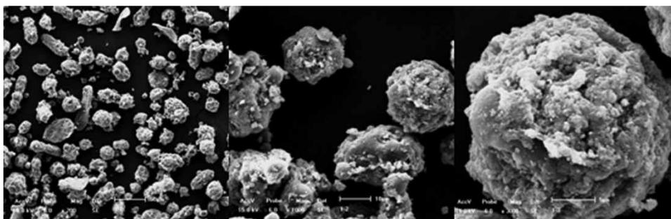
Figure 1 | SEM images of CS/EPTAC/Fe<sub>3</sub>O<sub>4</sub>.
