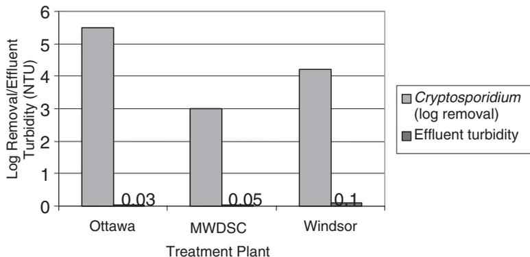
**Figure 2** *Cryptosporidium* removals and effluent turbidity values under stable operating conditions
