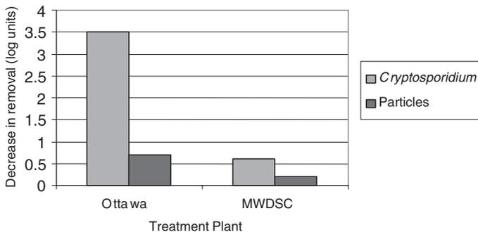
**Figure 4** Decreases in *Cryptosporidium* and particle removals during breakthrough
