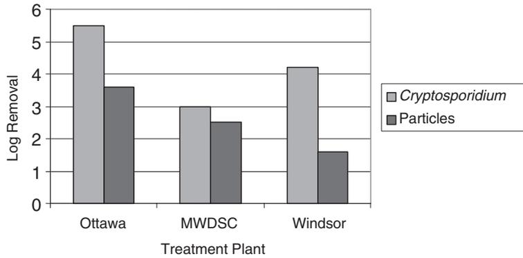
**Figure 1** Removals of *Cryptosporidium* and particles under stable operating conditions
