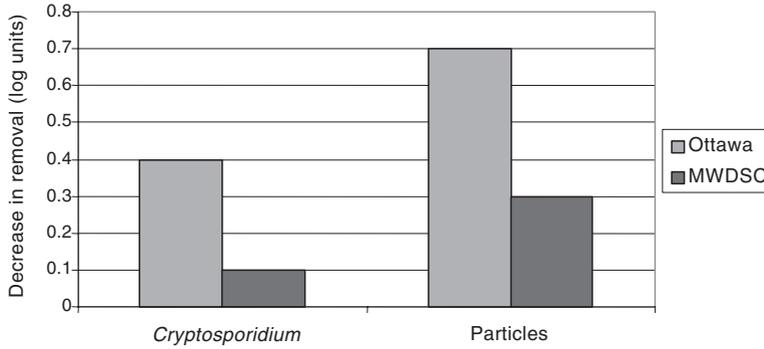
**Figure 3** Decreases in removals of *Cryptosporidium* and particles during ripening
