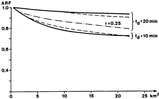
Fig. 6. Observed *ARF* (solid lines) and *M-ARF* determined for lateral distribution ratio  $r=0.5$  (broken lines) for 10 min duration (two lower graphs) of event 1 of the storm events presented by Niemczynowicz and Jönsson (1981), and for 20 min duration (three upper graphs) also *M-ARF* with  $r=0.25$ , i.e.  $k$  in Eq. (7) kept at the same value as for the 10 min. storm, as indicated on the graph.
