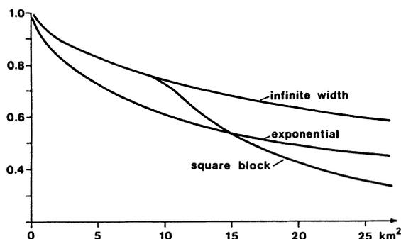
Fig. 5. *M-ARF* for block rain of 10 min duration assuming different intensity distributions transverse to the storm movement: infinite width, square block distribution, exponential intensity distribution with  $r = 0.7$ . Storm speed 5 m/s.
