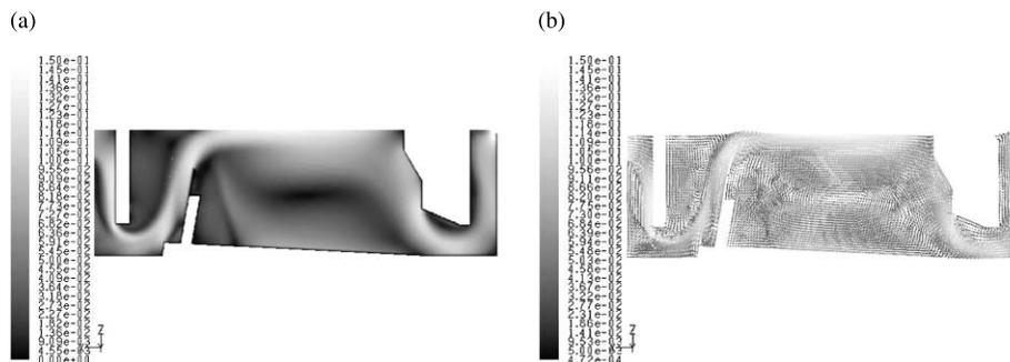
**Figure 3** | (a) Velocity contours +500 mm extended baffle; (b) velocity vectors +500 mm extended baffle.
