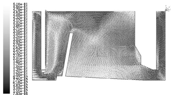
**Figure 9** | Velocity vectors at 4.0 m depth.
