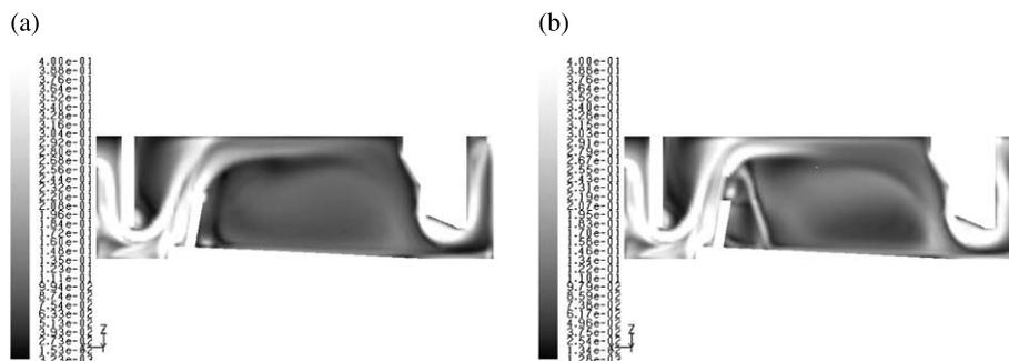
**Figure 4** | (a) Vortex contours; (b) vortex contours +500 mm extended baffle.
