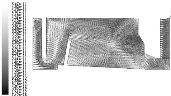
**Figure 7** | Velocity vectors at 2.9 m depth.
