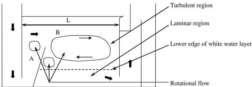
**Figure 1** | Typical DAF design. 'A', the 'contact zone' where hydraulic retention times (HRT) are typically 60–240 seconds and rates are 20–110 m<sup>3</sup> h<sup>-1</sup>; 'B', generally referred to as the 'clarification zone' where the upper cross-flow velocities are generally <0.05 m s<sup>-1</sup> including any circulation currents; loading rates are a function of influent and tank dimensions, i.e. length (L) and width.
