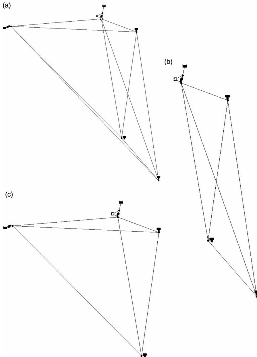
**Figure 5** | Illustrating an adaptation to structural changes in water network. (a) EPANET Net 3 after standard model reduction. (b) EPANET Net 3 simplified model layout when Pump 10 was removed. (c) EPANET Net 3 simplified model layout when Tank 2 was removed.
