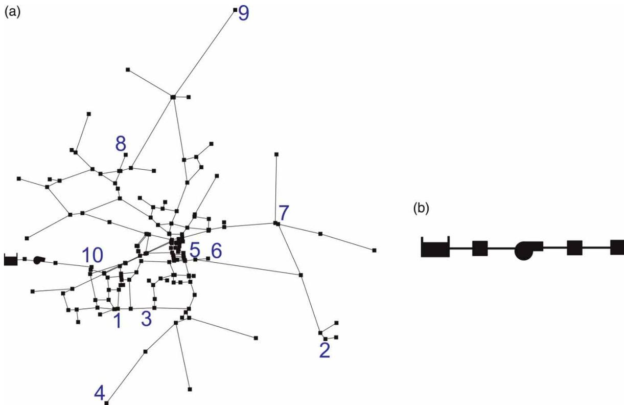
**Figure 9** | The water network model before (a) and after (b) the simplification. Numbers indicate a single node to be retained, varied in elevation with reference to the reservoir and in location in the water network.
