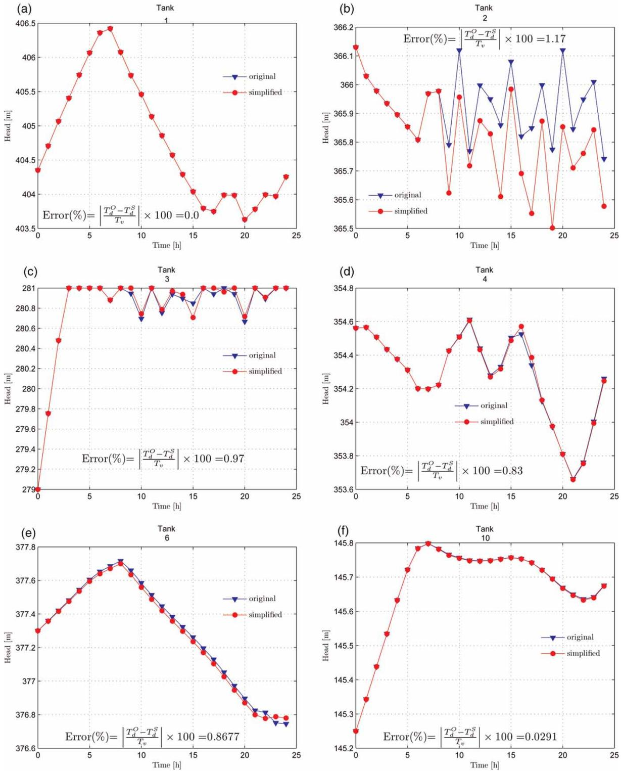
**Figure 6** | Comparison of simulated tank trajectories for water networks from Table 4. (a) Simulated trajectories for Tank 1 from Network 1. (b) Simulated trajectories for Tank 2 from Network 2. (c) Simulated trajectories for Tank 3 from Network 2. (d) Simulated trajectories for Tank 4 from Network 2. (e) Simulated trajectories for Tank 6 from Network 3. (f) Simulated trajectories for Tank 10 from Network 3.
