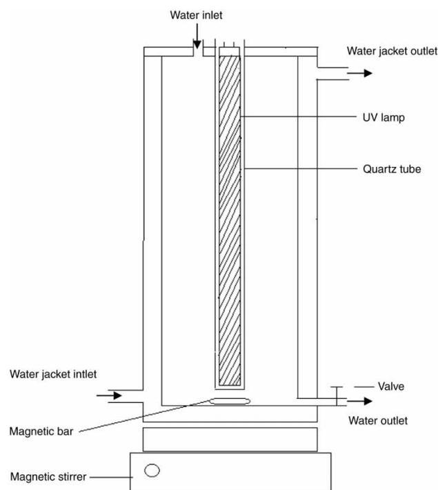
Figure 1 | Schematic diagram of the ultraviolet (UV) reactor.
