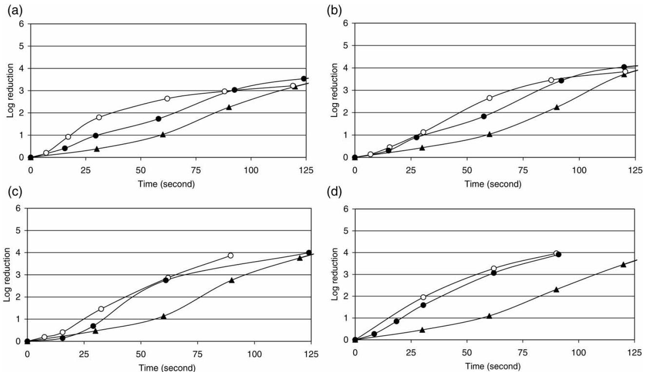
**Figure 4** | Bacterial reduction by the UV and the UV/H<sub>2</sub>O<sub>2</sub> processes in waters containing 6 mg l<sup>-1</sup> fulvic acid. (a) H<sub>2</sub>O<sub>2</sub> = 0 mg l<sup>-1</sup>, (b) H<sub>2</sub>O<sub>2</sub> = 10 mg l<sup>-1</sup>, (c) H<sub>2</sub>O<sub>2</sub> = 25 mg l<sup>-1</sup>, and (d) H<sub>2</sub>O<sub>2</sub> = 50 mg l<sup>-1</sup>; key: ○— *Escherichia coli*, ●— *Pseudomonas aeruginosa*, ▲— *Bacillus subtilis*.
