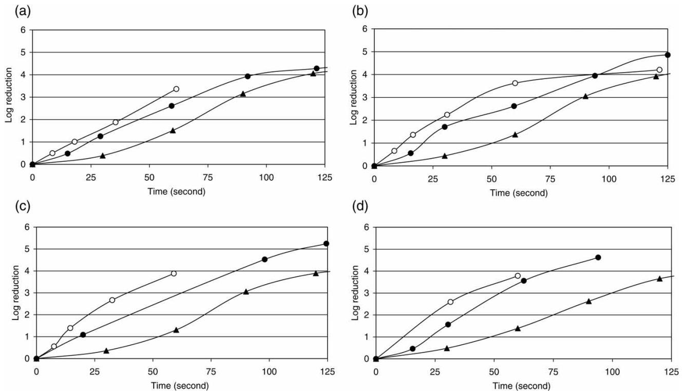
**Figure 2** | Bacterial reduction by the UV and the UV/H<sub>2</sub>O<sub>2</sub> processes in waters containing 0 mg l<sup>-1</sup> fulvic acid. (a) H<sub>2</sub>O<sub>2</sub> = 0 mg l<sup>-1</sup>, (b) H<sub>2</sub>O<sub>2</sub> = 10 mg l<sup>-1</sup>, (c) H<sub>2</sub>O<sub>2</sub> = 25 mg l<sup>-1</sup>, and (d) H<sub>2</sub>O<sub>2</sub> = 50 mg l<sup>-1</sup>; key: ○— *Escherichia coli*, ●— *Pseudomonas aeruginosa*, ▲— *Bacillus subtilis*.
