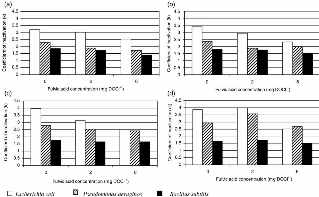
**Figure 5** | Comparison of inactivation coefficients for *E. coli*, *P. aeruginosa* and *B. subtilis* spores in disinfected water containing various concentrations of fulvic acid. (a) H<sub>2</sub>O<sub>2</sub> = 0 mg l<sup>-1</sup>, (b) H<sub>2</sub>O<sub>2</sub> = 10 mg l<sup>-1</sup>, (c) H<sub>2</sub>O<sub>2</sub> = 25 mg l<sup>-1</sup>, and (d) H<sub>2</sub>O<sub>2</sub> = 50 mg l<sup>-1</sup>. DOC, dissolved organic carbon.
