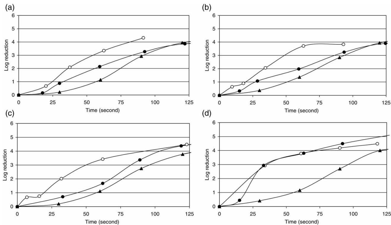
**Figure 3** | Bacterial reduction by the UV and the UV/H<sub>2</sub>O<sub>2</sub> processes in waters containing 2 mg l<sup>-1</sup> fulvic acid. (a) H<sub>2</sub>O<sub>2</sub> = 0 mg l<sup>-1</sup>, (b) H<sub>2</sub>O<sub>2</sub> = 10 mg l<sup>-1</sup>, (c) H<sub>2</sub>O<sub>2</sub> = 25 mg l<sup>-1</sup>, and (d) H<sub>2</sub>O<sub>2</sub> = 50 mg l<sup>-1</sup>; key: ○—*Escherichia coli*, ●—*Pseudomonas aeruginosa*, ▲—*Bacillus subtilis*.
