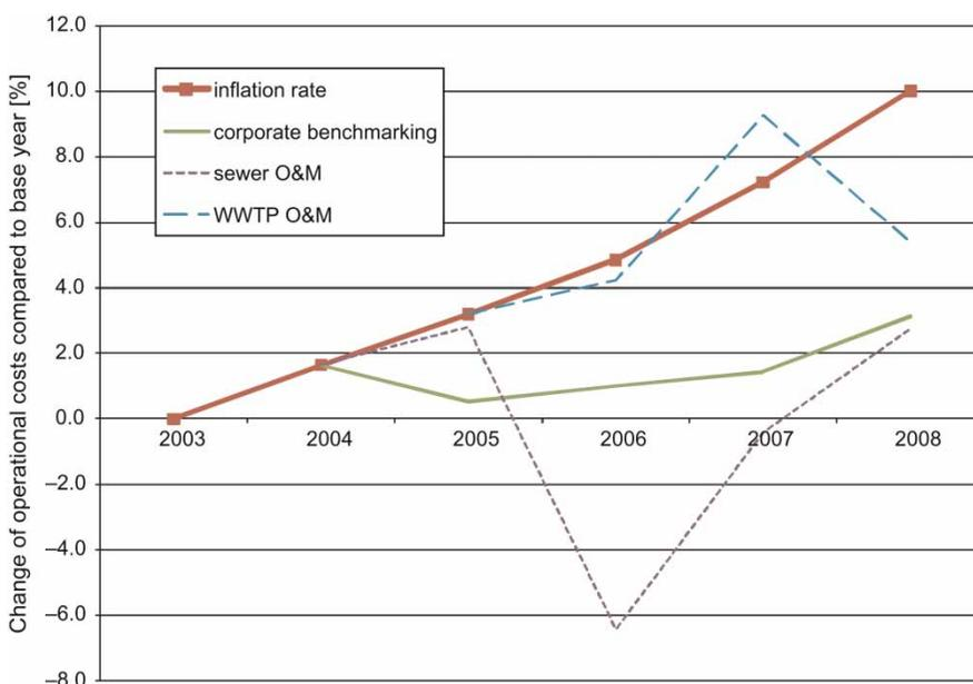
**Figure 3** | Average cost increase in different analysed benchmarking objects (12 utilities).
