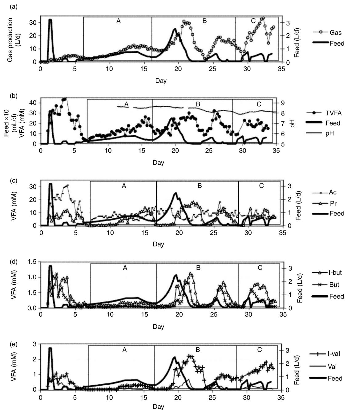
**Figure 2** | Online measuring results from propionate control experiment by regulating the feed flow rate: (a) biogas production, (b) total VFA and pH, (c) acetate and propionate, (d) iso-butyrate and butyrate, (e) iso-valerate and valerate.
