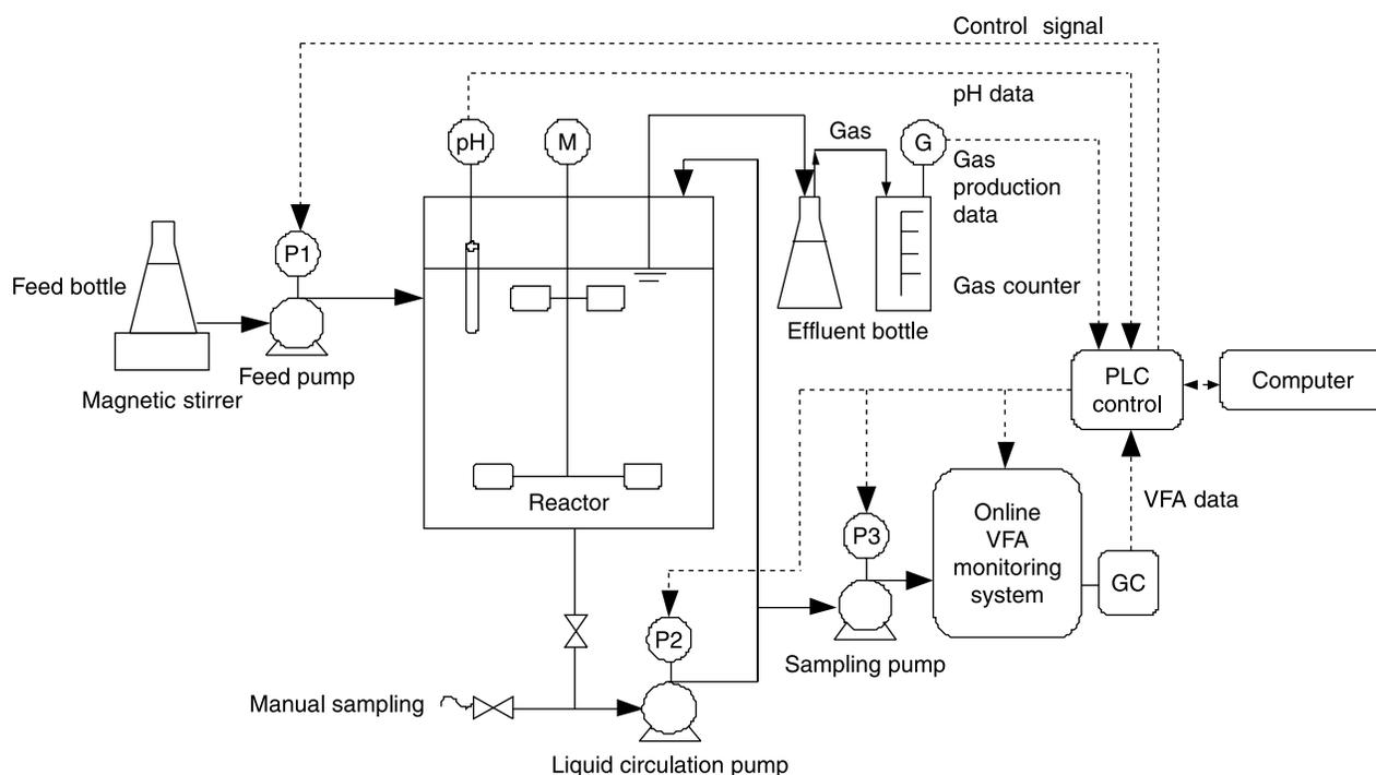
Figure 1 | Diagram of experimental setup.
