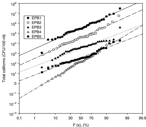
**Figure 3** | Probability distribution of total coliforms at the WRP of Empuriabrava.
