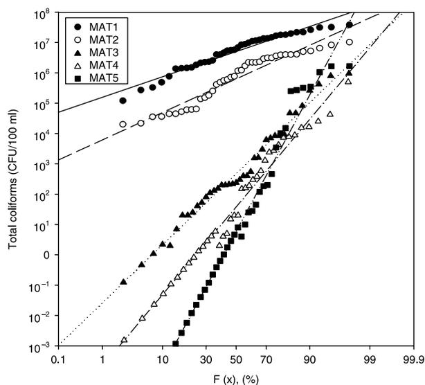
**Figure 5** | Probability distributions of total coliforms at the WRP of Mataró.
