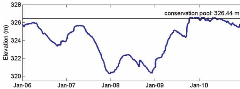
Fig. 3. Diagram showing the stage variation of Lake Lanier from 2006–11 (Anonymous, 2013). Note the extremely low stage of the lake during the critical part of 2008.
