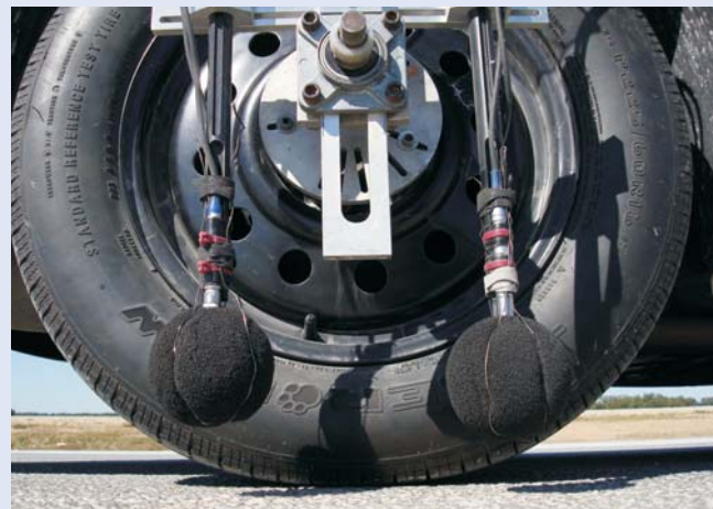
Figure 1. On-board sound intensity is a standardized method for evaluating the intensity of noise due to the interaction of tire and pavement. Tests are typically conducted at 60 mph. Visible here are OBSI's two probes; each has a pair of microphones surrounded by a windscreen. The two probes allow engineers to measure noise emanating from both the front and the back of the contact patch where the tire meets the road.
