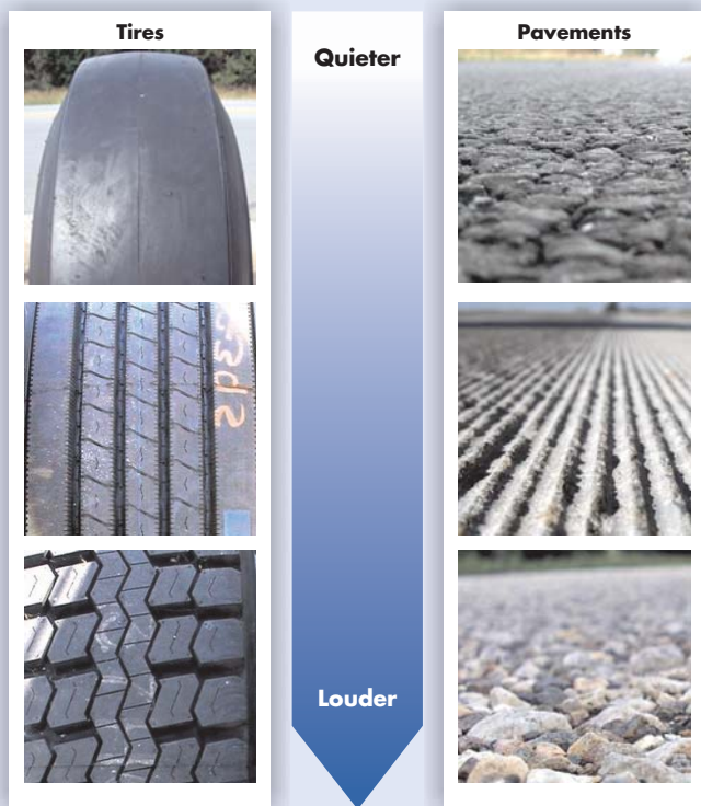
Figure 2. Tires and pavements both contribute to road noise. Tires without tread can be very quiet. Those with simple geometries can be modestly louder, but those with large, blocky tread patterns are among the loudest. The quietest pavements include those with fine texture and significant porosity. Those without porosity but with fine texture can be somewhat louder. Pavements with large or worn textures are among the loudest. All three pavement photos show a sample that is a few centimeters across.
