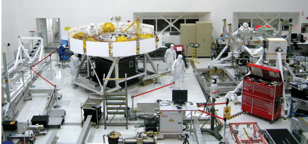
ONE OF THE LARGEST CLEAN ROOMS IN THE WORLD is at NASA's Jet Propulsion Laboratory in California. The specially clothed technicians here are working on the Mars Curiosity rover. (Photo courtesy of Yvette Cendes.)
