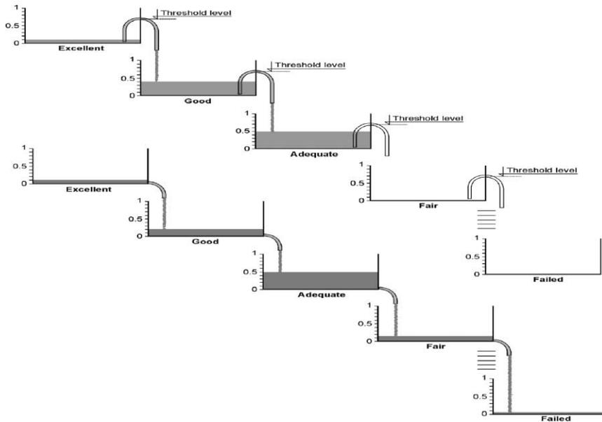
**Figure 4** | Visualization of threshold effects: bottom reservoirs – analogous to traditional Markov process (no thresholds); top reservoirs – analogous to deterioration curves with thresholds.
