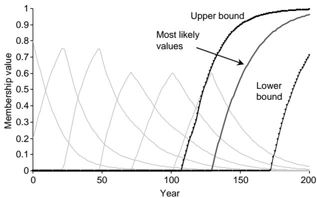
**Figure 8** | Deterioration curves with fuzzy confidence band ( $\alpha = [0.9\max(\mu_t^{D_1}, \mu_t^{D_2}, \dots, \mu_t^{D_7})]$ ) for the 'failed' state.
