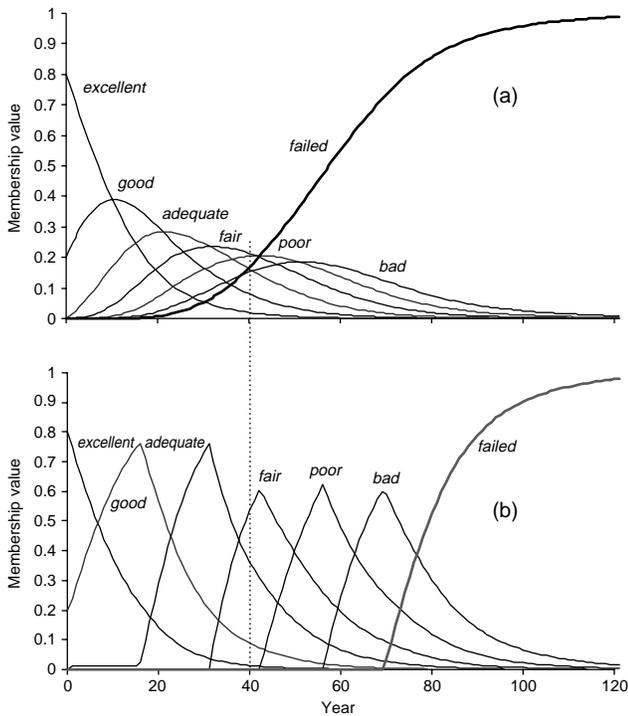
**Figure 3** | Deterioration curves without (a) and with (b) membership threshold parameters.
