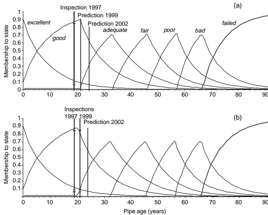
Figure 6 | Model validation with (a) one inspection in 1997 and (b) two inspections in 1997 and 1999.
