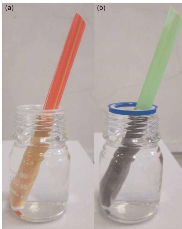
**Figure 4** | Testing of water disinfection by nanosilver textile kits: (a) yellowish textile kit, (b) grayish textile kit.
