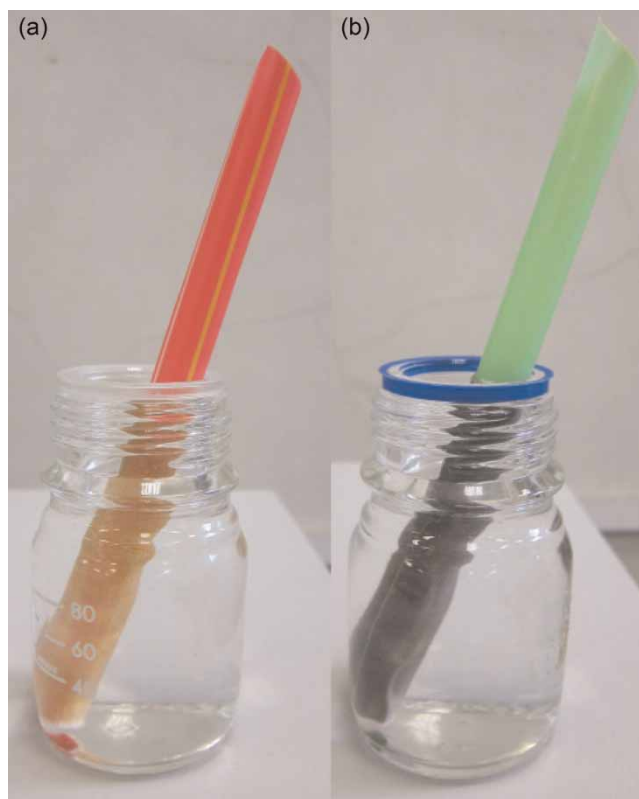
Figure 4 | Testing of water disinfection by nanosilver textile kits: (a) yellowish textile kit, (b) grayish textile kit.
