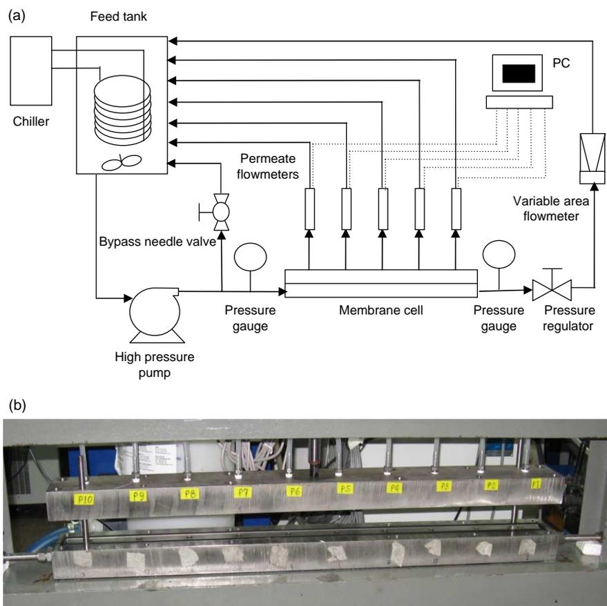
**Figure 1** | (a) Schematic diagrams of the RO setup and (b) the picture of the 1-m long RO membrane cell.
