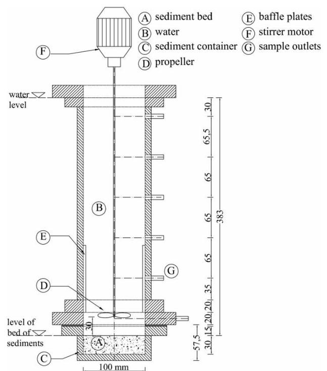
Figure 1 | Erosion meter device.
