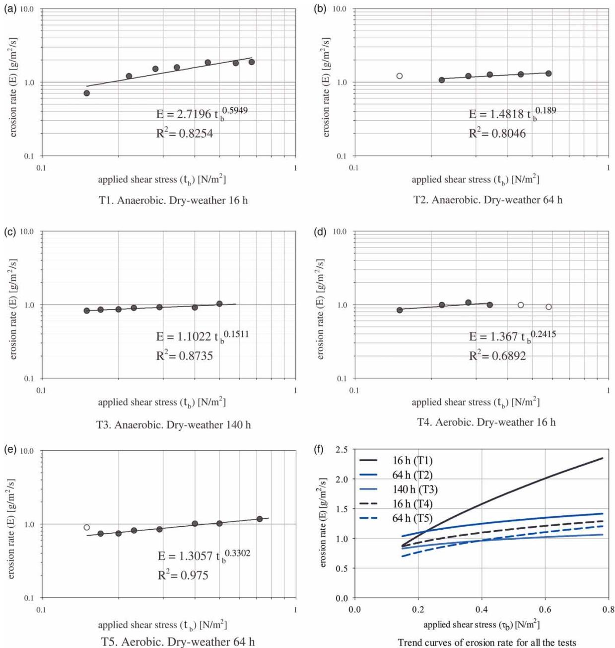
**Figure 3** | (a) to (e) Erosion rate against applied shear stress during tests under anaerobic (T1–T3) and aerobic (T4–T5) conditions. Double log plot and best fitting-trend curves (power trend). (f) Power trend lines obtained for T1 to T5 are shown comparatively.
