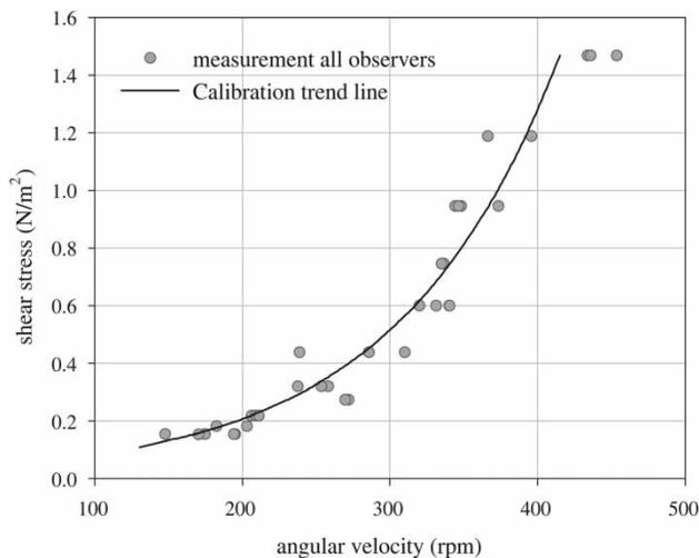
**Figure 2** | Erosionmeter calibration curve. Shear stress against angular velocity and second-order trend curve.
