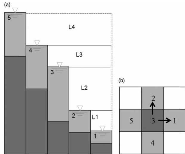
**Figure 1** | (a) Cells ordered in NH according to their ranks, L1–L4 are layers of free spaces between the water levels of two cells that are available within NH for water distribution, the numbers shown are cell ranks. In this diagram the ground level for each cell is shown in dark grey and the water level light grey, (b) an example of outflow fluxes (shown by arrows) from the central cell having rank 3 to its neighbouring cells.
