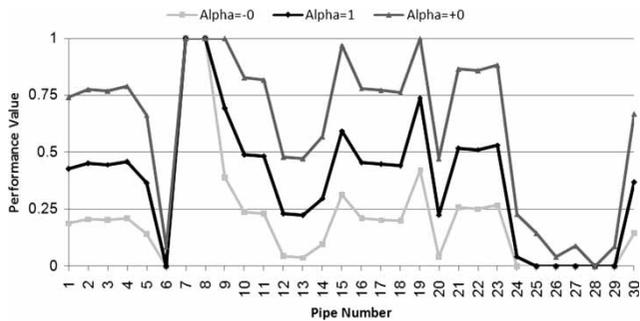
**Figure 9** | Performance value of different pipes in terms of self-cleaning velocity at beginning of design period (2010);  $\alpha$ -levels of 1 and 0 (– and + refer to lower and upper bounds, respectively).
