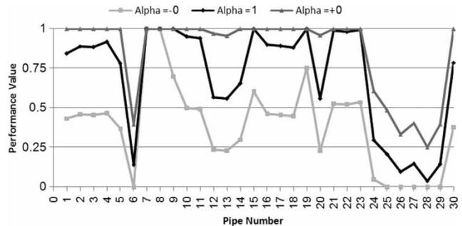
**Figure 13** | Performance value of different pipes in terms of velocity under maximum discharge ( $Q_{max}$  in 2035);  $\alpha$ -levels of 1 and 0 (– and + refer to lower and upper bounds, respectively).
