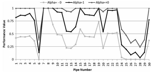
**Figure 11** | Performance value of different pipes in terms of self-cleaning velocity at end of design period (2035);  $\alpha$ -levels of 1 and 0 (– and + refer to lower and upper bounds, respectively).
