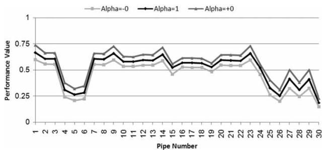
**Figure 10** | Performance value of different pipes in terms of relative depth under self-cleaning discharge ( $Q_{sc}$ ) at beginning of design period (2010);  $\alpha$ -levels of 1 and 0 (– and + refer to lower and upper bounds, respectively).
