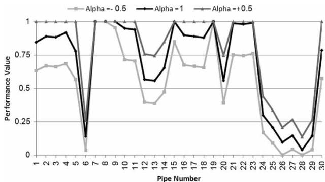
**Figure 15** | Performance value of different pipes in terms of velocity under maximum discharge ( $Q_{max}$  in 2035);  $\alpha$ -levels of 1 and 0.5 (– and + refer to lower and upper bounds, respectively).
