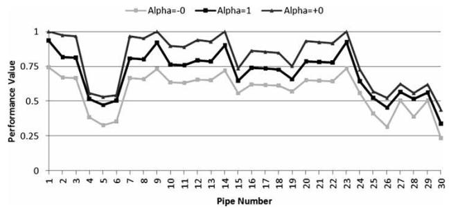
**Figure 12** | Performance value of different pipes in terms of relative depth under self-cleaning discharge ( $Q_{sc}$ ) at end of design period (2035);  $\alpha$ -levels of 1 and 0 (– and + refer to lower and upper bounds, respectively).
