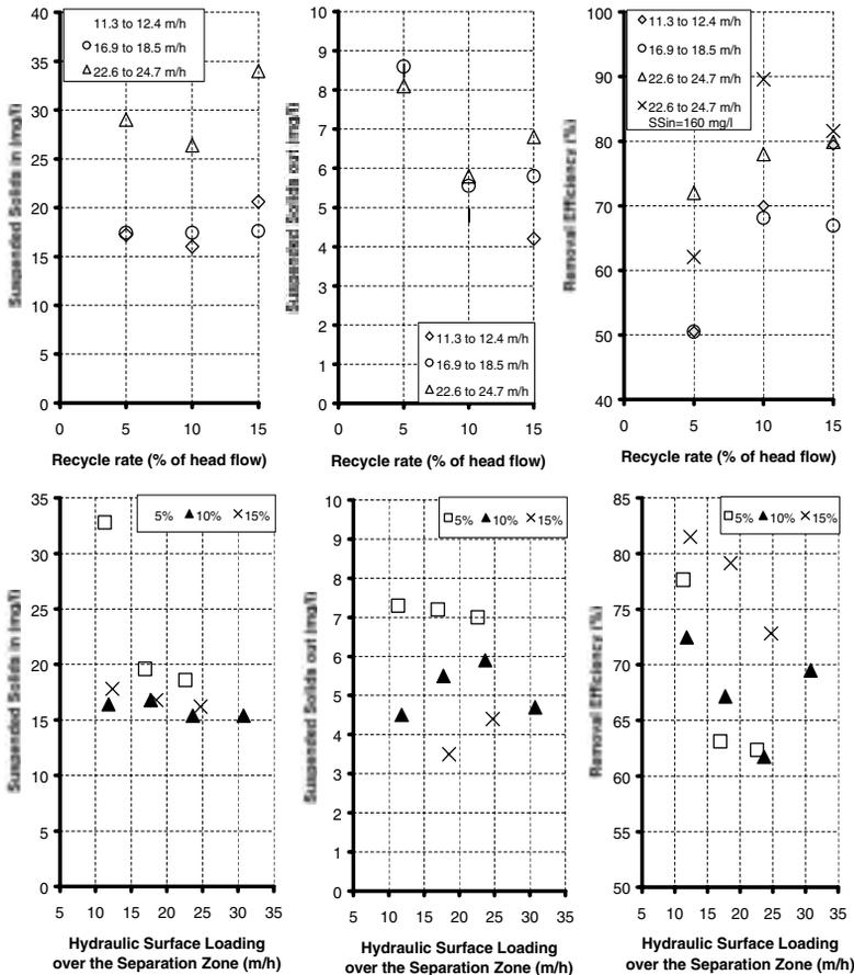
**Figure 6** Increase of recycle rate for constant hydraulic surface loading /top/ and increase of hydraulic surface loading for constant recycle rate /bottom/. The case with high concentration of incoming SS of approximately 160 mg SS/l is only shown as removal efficiency for readability reasons
