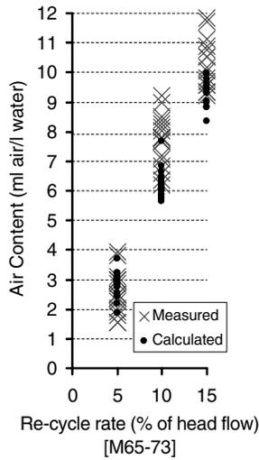
**Figure 5** Measured and calculated air content in the contact zone at Sjölanda WWTP
