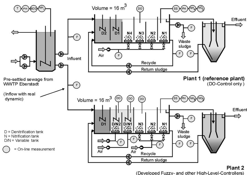
**Figure 1** Schematic flow diagram of the wastewater treatment pilot plant
