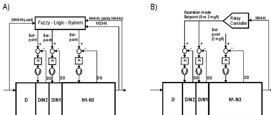
**Figure 2** Block diagrams of high-level fuzzy-controllers (A) and conventional relay controller (B)
