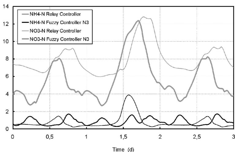
**Figure 4**  $\text{NH}_4\text{-N}$  and  $\text{NO}_3\text{-N}$  effluent concentrations for fuzzy-controller variant N3 and the conventional relay controller (simulation results)
