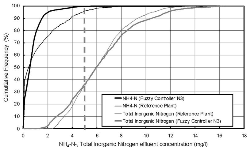
**Figure 5** Cumulative frequency of  $\text{NH}_4\text{-N}$  and total inorganic nitrogen effluent concentrations (experimental results)
