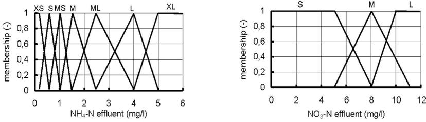
**Figure 3** Membership-functions in the high-level fuzzy-controllers for the input variables  $\text{NH}_4\text{-N}$ - and  $\text{NO}_3\text{-N}$ -concentration in the effluent
