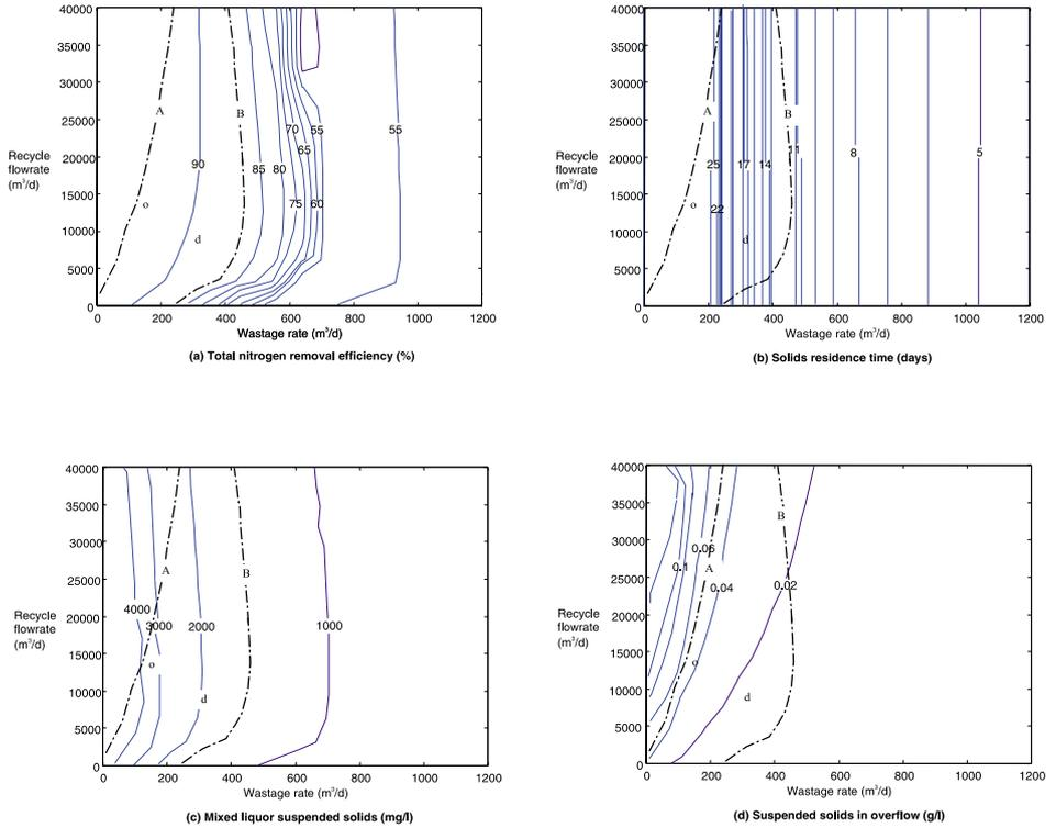
**Figure 4** The operating space diagrams for the base case design (A = solids constraint, B = constraint of effluent total nitrogen, o = optimal operation for nitrogen removal, d = design point)
