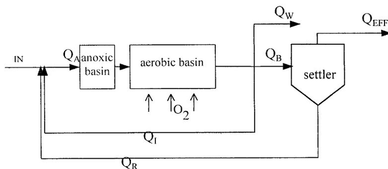
**Figure 3** The modified Ludzack-Ettinger process
