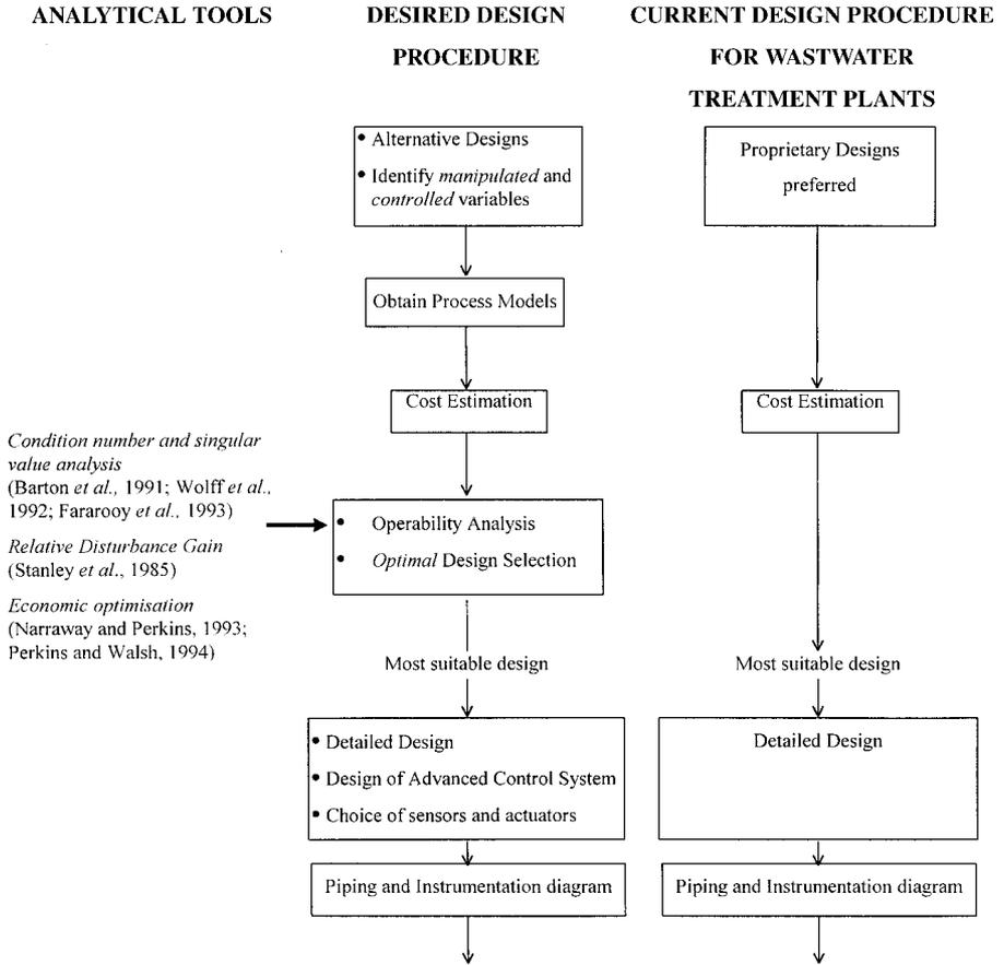
**Figure 1** Methodology for integrating process design and control showing the difference between the desired methodology and that generally used by wastewater design engineers
