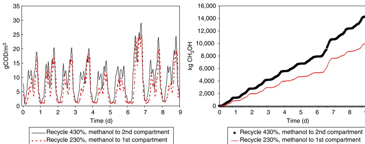
**Figure 4** | Readily biodegradable COD ( $S_s$ ) at the end of anoxic phase (gCOD/m<sup>3</sup>, left), i.e. carried over to aerobic phase and thus of no use for denitrification, and the respective cumulative amounts of  $S_s$  (methanol equivalent, right) with two sets of operational settings. Total nitrogen removal rate 70% and  $T = +10^\circ\text{C}$  in both cases.
