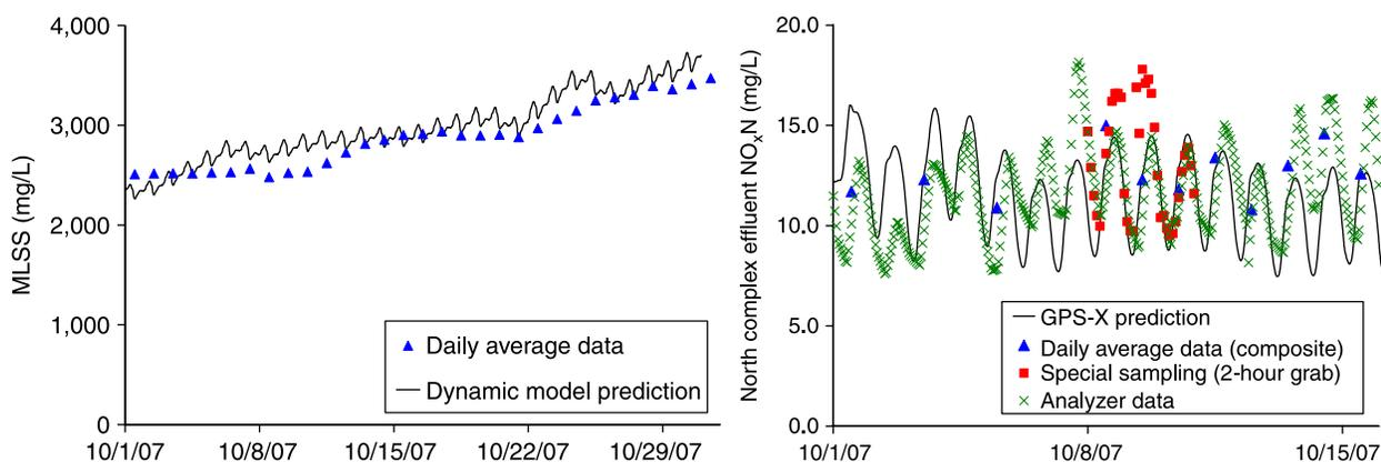
Figure 1 | Calibration results—MLSS concentration (left), and effluent NO<sub>x</sub>N (right).
