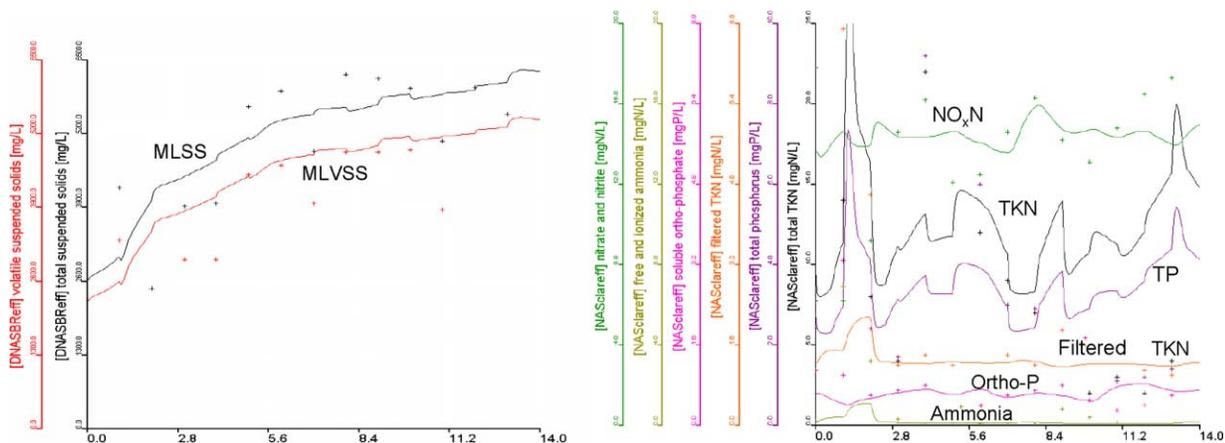
**Figure 5** | Illustration of calibration for DNAS bioreactor MLSS and MLVSS (left) and NAS clarifier effluent nutrients (right).
