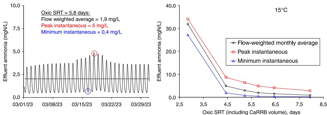
**Figure 2** | Selecting a design SRT using a 'wedding cake' analysis (left) and plotting the peak, average and minimum effluent ammonia concentrations for several SRTs (right).
