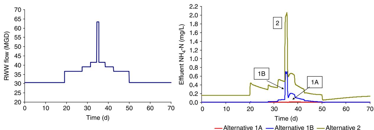
**Figure 6** | Basis of dynamic simulations for raw wastewater flow (left), and dynamic model response of ammonia for alternatives 1A, 1B, and 2 (right).
