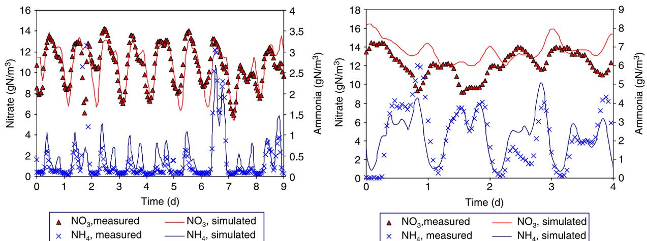
**Figure 3** | Simulated and measured ammonium and nitrate nitrogen at the end of aeration line for model calibration (left,  $T = +19^{\circ}\text{C}$ ) and validation (right,  $T = +9^{\circ}\text{C}$ ).
