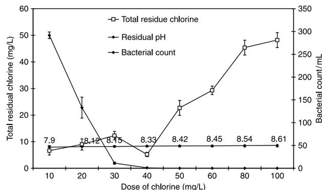
Figure 5 | Break point chlorination of UAFFR effluent.
