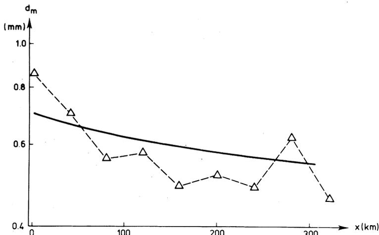
Fig. 4. The distribution of the median diameter along the lower river Niger, theoretical compared with measured. The following data are used:  $d_{m\bar{\sigma}} = 0.7$  mm,  $q = 10.6$  m<sup>2</sup>/s,  $I_0 = 1.07 \cdot 10^{-4}$ ,  $\alpha = 1.38 \cdot 10^{-6} \text{m}^{-1}$ .
