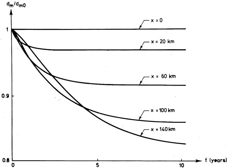
Fig. 1. Variation of the median grain diameter with time and space.
