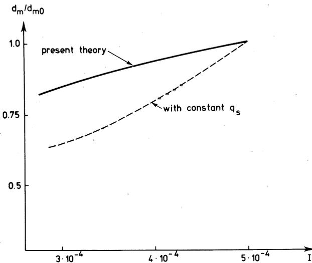
Fig. 3. The median diameter,  $d_m$ , as a function of the slope (same data as in Fig. 1). The relation shown by the dotted line is not stationary for a given longitudinal river profile.
