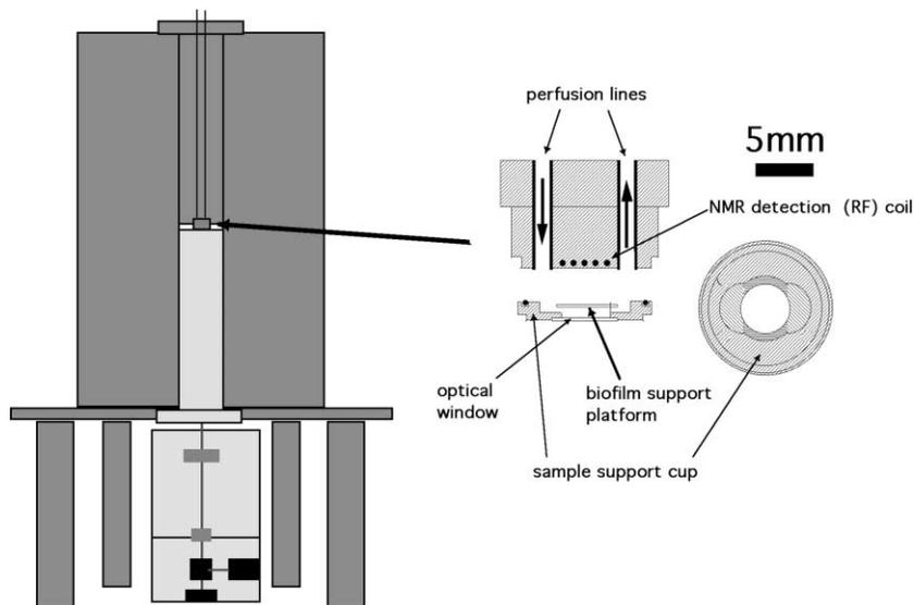
**Figure 1** Left: diagram for the combined optical and magnetic resonance microscope, consisting of an actively shielded 11.7 T wide-bore magnet with top-loading NMR and bottom-loading optical components with the perfused sample chamber at their interface. Right: expanded and exploded side and top-down view of the sample chamber containing the glass cover slip sample support
