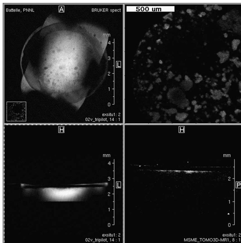
**Figure 2** Sequential MRI and confocal images acquired for a sparse, early biofilm. Top left: water-selective top-down MRI of the coverslip with corresponding confocal image in the inset; top right: expanded view of the confocal image (same as inset); bottom left: water-selective side-view MRI (the dark rectangle is the cross-section of the cover slip); bottom right: biofilm-selective MRI (40  $\mu\text{m}$  thick side-view plane from 3D-MRI measurement)
