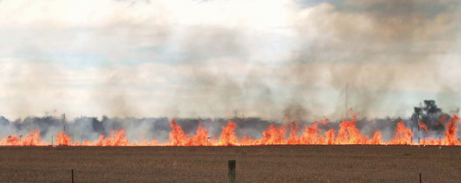
FIGURE 2. TOWERS AND TROUGHS, IN REALITY. In this experimental grass fire, the few visible peaks are separated by gaps in which the wind currents sweep downward between the flames and feed the peaks on opposite sides. (Courtesy of Mark Finney, US Forest Service, Missoula Fire Sciences Laboratory.)
