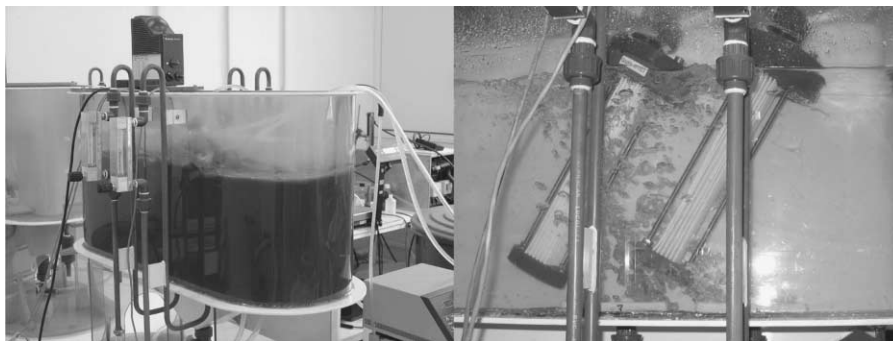
Figure 1 Pilot bioreactor and membranes used for the experiments
