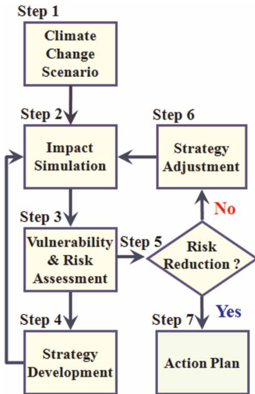
Figure 1 | Process for developing and adjusting strategies.
