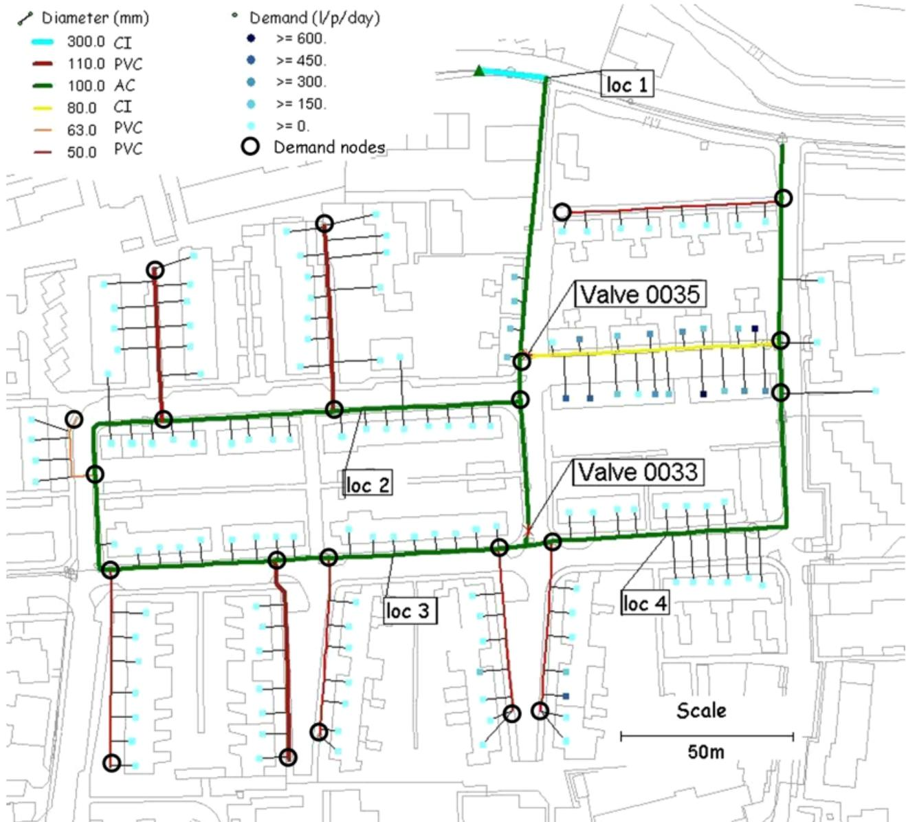
**Figure 1** | Network layout. Water enters at location 1; a continuous demand of 400 L/h was extracted at loc. 4. Valves 0033 and 0035 are closed in the branched layout and open in the looped layout. Valve 0035 is placed at the 80 mm CI main.
