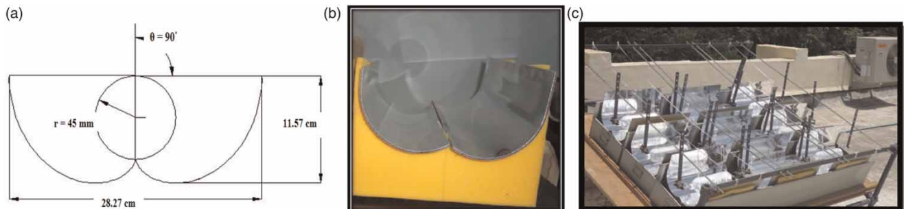
Figure 1 | Details of the CPC system: (a) dimensions, (b) single CPC, (c) support system for the CPCs.
