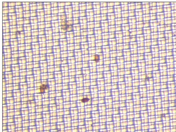
**Figure 5** | Close view of *Trichuris suis* eggs blocked on a 10  $\mu\text{m}$  pore size filter cloth. Note that the threads in the filter cloth have a thickness of approx. 35  $\mu\text{m}$  and therefore are thicker than the 10  $\mu\text{m}$  openings. This gives an approx. 5% open area in the filter cloth. The picture was taken by optical microscope and subsequently enlarged.
