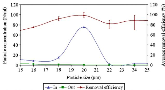
**Figure 4** | Particle size distribution in the inlet of the drumfilter and outlet flows and removal efficiency for particle sizes within 15 and 25  $\mu\text{m}$ , as a function of particle size. Each size interval in the figure is represented by its average size. Error bars indicate the maximum and minimum values of the removal efficiency.
