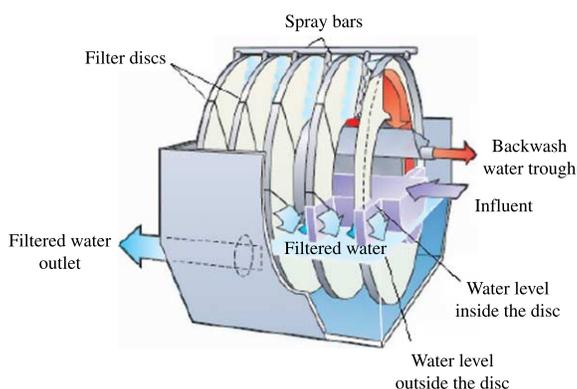
Figure 1 | The discfilter process flow diagram (Quinzaños 2006).
