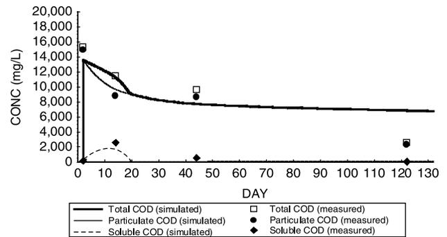
Figure 8 | COD Concentrations versus Time in WAS Tests (Scenario 2).
