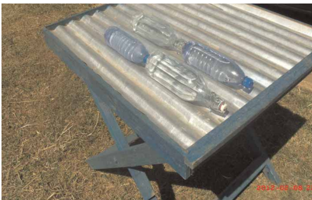
Figure 2 | Clear shallow well water in PET plastic and swing top glass bottles during exposure to direct sunlight at Makerere University, Kampala.
