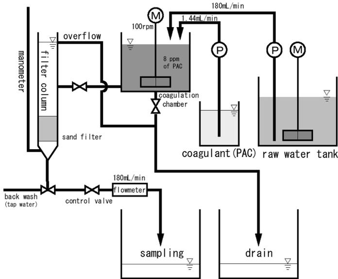
**Figure 1** Schematic of the experimental set up
