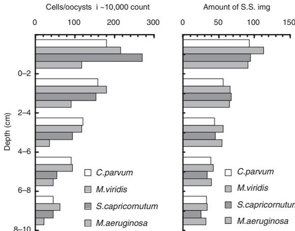
**Figure 5** Amount of suspended solid and cell/oocyst counts captured in the sand filter
