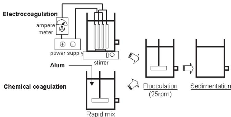
**Figure 1** The experimental set-up
