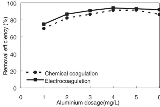
**Figure 2** Effect of aluminium dosage on the removal efficiency
