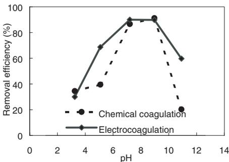
**Figure 3** Effect of pH on turbidity removal efficiency
