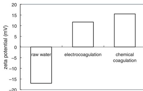
**Figure 5** The zeta potential after electrolysis and rapid mix respectively
