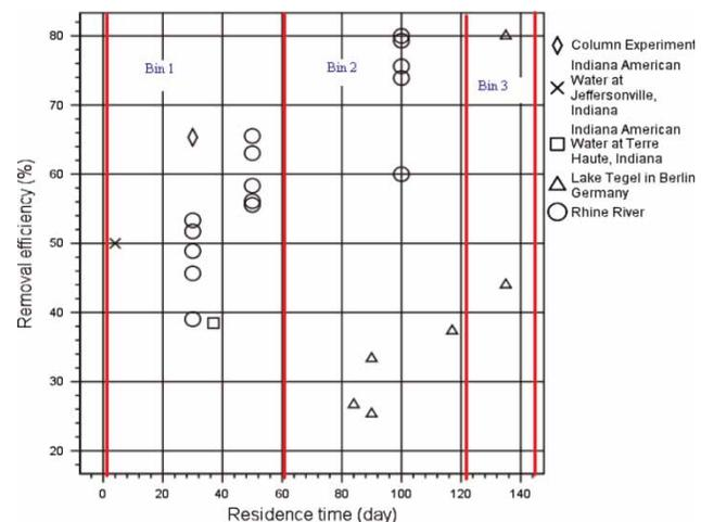
Figure 1 | Scatter plot of DOC removal efficiency versus residence time for BF systems.
