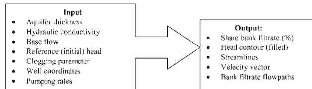
Figure 4 | NASRI BF simulator data input and output parameters.
