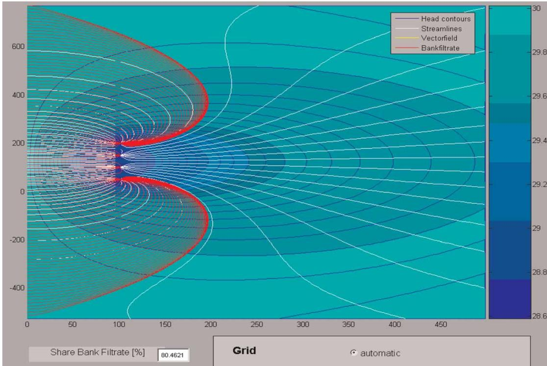
**Figure 5** | Sample NASRI BF Simulator output display (4 wells 100 m from bank 50 m well spacing C/C, hydraulic conductivity 0.006 m/s).
