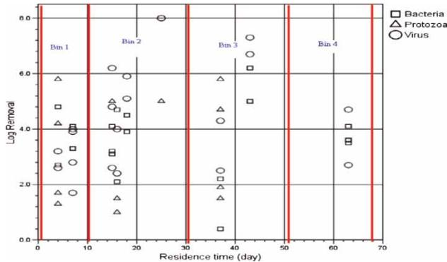
**Figure 2** | Scatter plot of microbes removal efficiency versus residence time for BF systems.
