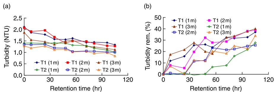
**Figure 5** Turbidity and particle removal rate in rainfall Case 3. (a) Turbidity and (b) Turbidity removal rate
