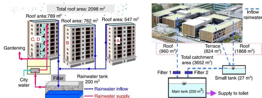
**Figure 1** Schematic diagram of rainwater storage and supply systems at SNU
