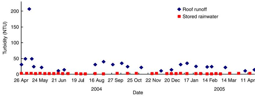
**Figure 2** Turbidity of roof runoff and stored rainwater over a one-year period in a dormitory
