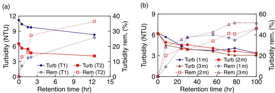
**Figure 4** Turbidity and particle removal rate in rainfall Case 1 and 2. (a) Case 1 and (b) T1 at case 2
