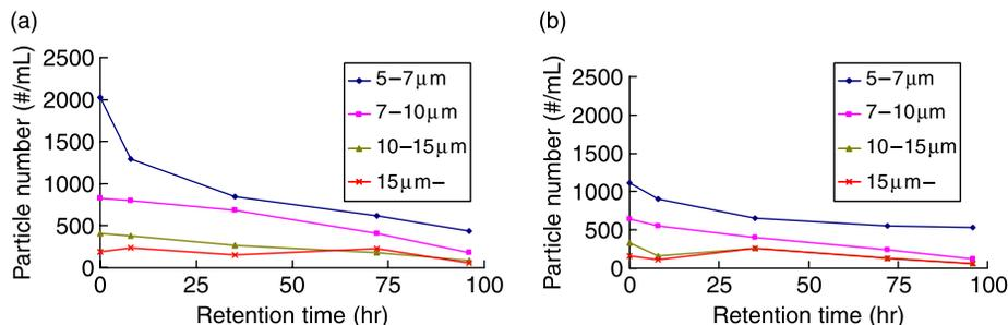
**Figure 6** Particle size distribution by size category in stored rainwater in T1, based on retention time in Case 3. (a) 1 m from bottom and (b) 3 m from bottom
