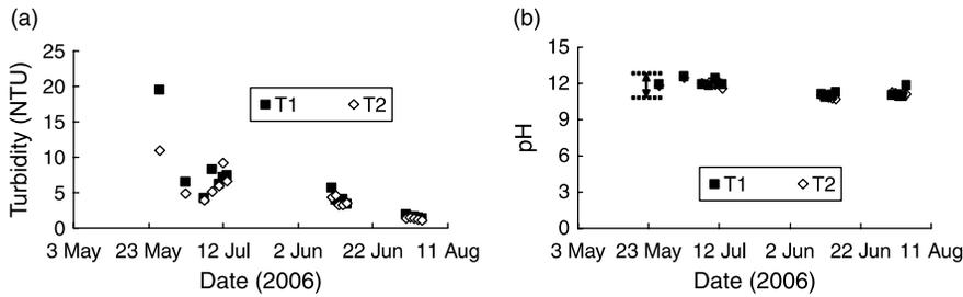
**Figure 3** Turbidity and pH of stored rainwater in the main tank of the Building #39. (a) Turbidity and (b) pH
