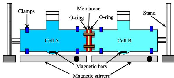
Figure 2 | Schematic diagram of experimental setup for diffusion tests.
