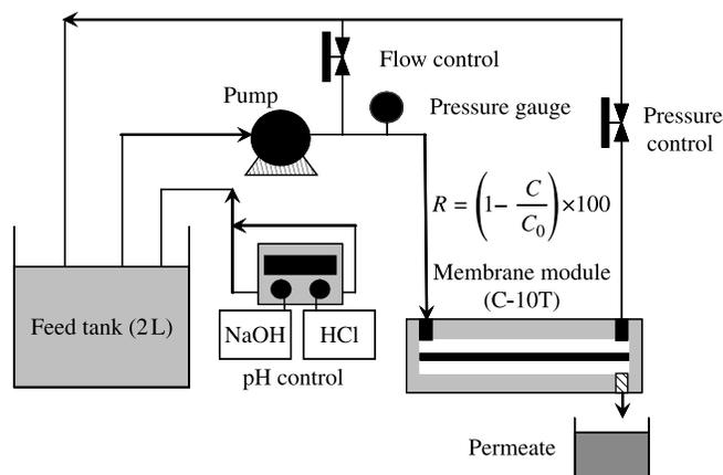
**Figure 1** | Schematic diagram of experimental setup for membrane efficiency tests.
