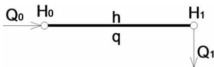
Figure 1 | Pipe with flows, heads, and head loss.
