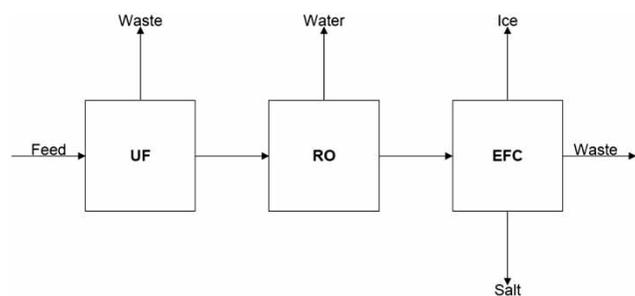
Figure 4 | The hybrid UF-RO-EFC process for the treatment of textile wastewater.
