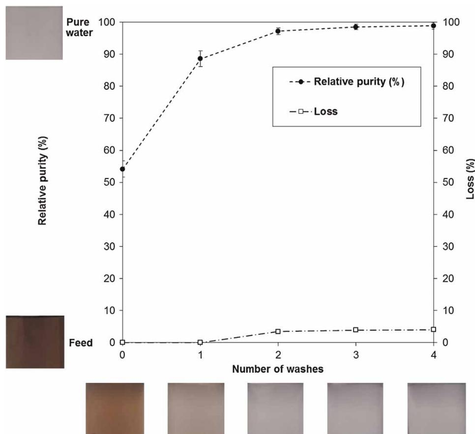
Figure 3 | Purity of ice product as a function of washing.
