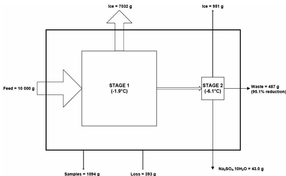
Figure 2 | Mass balance for the treatment of a textile wastewater using EFC.
