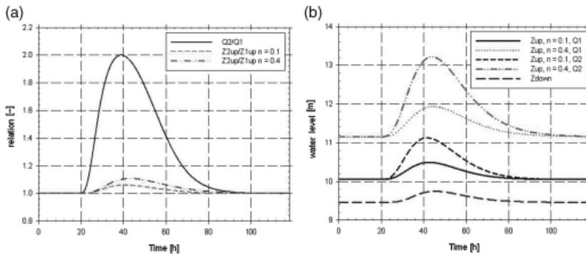
**Figure 9** | Influence of discharge and Manning coefficient ( $n = 0.4 \text{ m}^{-1/3} \text{ s}$  and  $n = 0.1 \text{ m}^{-1/3} \text{ s}$ ) on water levels. (a) shows the water level for varying discharge and Manning coefficient as a function of time. (b) depicts the relation between the discharge  $Q_1$  and  $Q_2$  used as upstream boundary condition and the resulting relation between the upstream water levels for different Manning coefficients.
