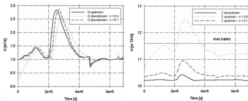
Figure 11 | Boundary conditions  $Q_{\text{upstream}}$  and calculated  $Q_{\text{downstream}}$  for  $n = 0.4 \text{ m}^{-1/3} \text{ s}$  and  $n = 0.1 \text{ m}^{-1/3} \text{ s}$  (left) and boundary conditions  $Z_{\text{downstream}}$  and calculated  $Z_{\text{upstream}}$  for  $n = 0.4 \text{ m}^{-1/3} \text{ s}$  and  $n = 0.1 \text{ m}^{-1/3} \text{ s}$  (right).
