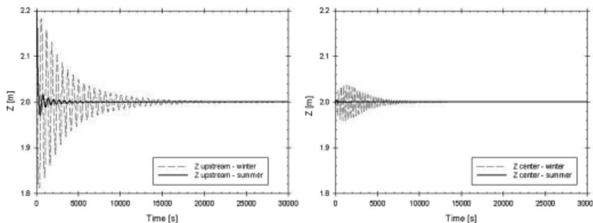
**Figure 4** | Upstream water level (left) and water level in the middle of the reach of 1400 m (right) for summer ( $n = 0.1 \text{ m}^{-1/3} \text{ s}$ ) and winter ( $n = 0.01 \text{ m}^{-1/3} \text{ s}$ ) conditions.
