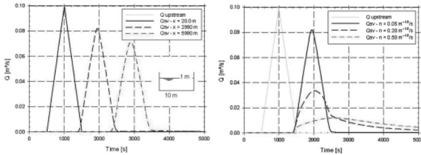
**Figure 6** | Numerical results of wave propagation by use of the Saint-Venant equations: result at different locations (left) and result at a single location ( $x = 2990$  m) for different values of the Manning coefficient  $n$  (right).
