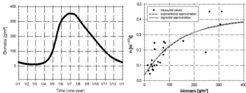
**Figure 3** | Variation of biomass density over the year (left) and relationship between Manning's roughness coefficient and biomass density according to a sigmoidal and an exponential approximation (right).
