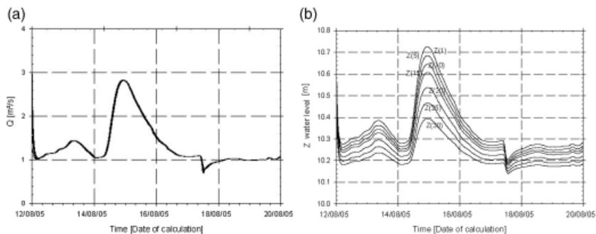
**Figure 12** | Calculation of discharge (a) and water level (b) at different sections of the River Aa. The discharge in seven sections hardly changes, while the water level decreases from upstream (1) to downstream (30).
