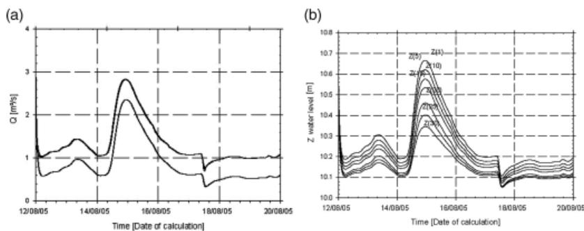
**Figure 13** | Calculation of discharge (a) and water level (b) at different sections of the River Aa, extracting a lateral outflow at a distance of 800 m (section 18). The discharge decreases in all sections downstream from section 18, while the water level decreases over the entire reach.
