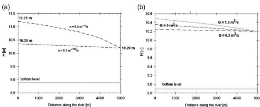
**Figure 10** | Backwater influence of the Manning coefficient on the water level for a given discharge of  $1 \text{ m}^3/\text{s}$  (left, (a)) and backwater influence of the discharge on the water level for a given amount of vegetation ( $n = 0.1 \text{ m}^{-1/3} \text{ s}$ ) (right, (b)).
