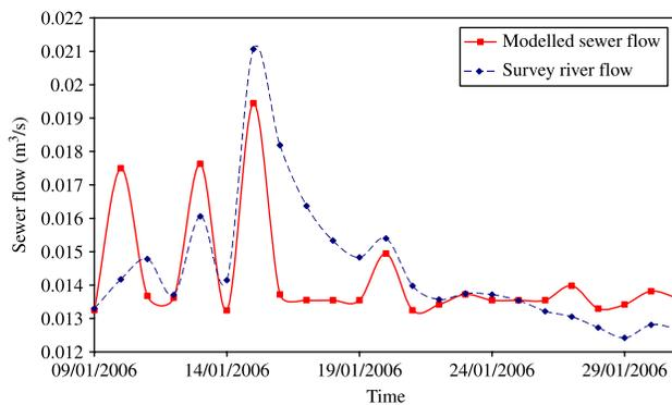
Figure 4 | Calibration hydrograph of the sewer network.
