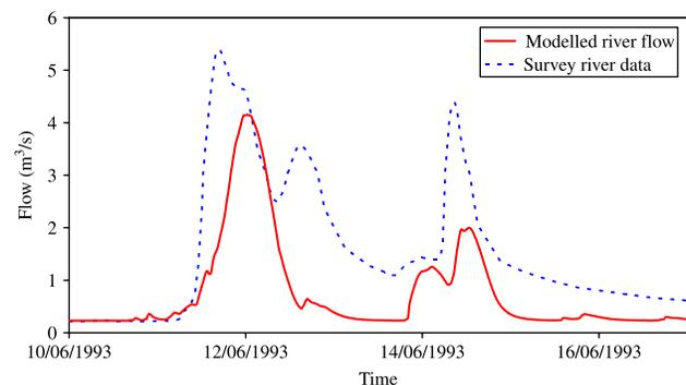
**Figure 3** | Calibration hydrograph at the Common's road river gauges in 1993.
