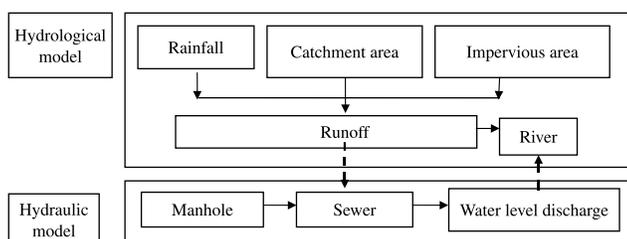
**Figure 2** | Interactions between various components of the modelling approach. (adapted from Mark et al. 2004).
