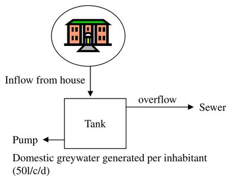
Figure 5 | A schematic of greywater use model.
