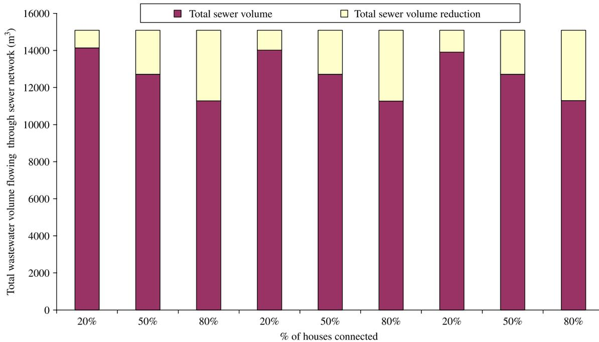
**Figure 6** | Simulated reduction of total daily sewer flow for each scenario.
