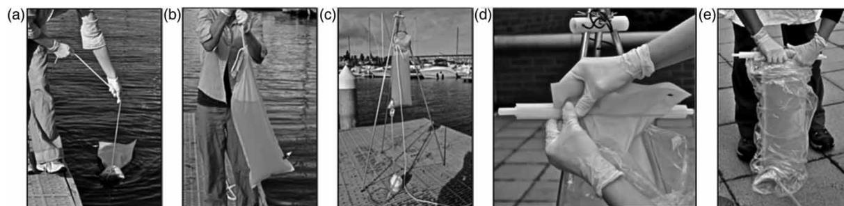
**Figure 1** | Photographs of sample collection and filtration. (a) Sample collection; (b) raise sample out of water; (c) hook sample on tripod stand and attach filter to port; (d) attach clamp to seal bag; (e) roll bag to force water through filter.
