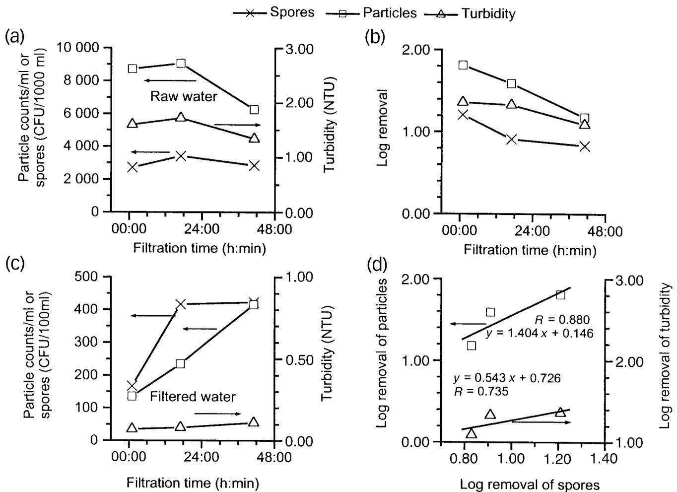
**Figure 7** | Monitoring the evolution of total particle count (2–150 μm), spores and turbidity, cycle No 585, Percol LT35, 0.16 to 0.24 mg/l, 96/12/16: (a) raw water, (b) log removal, (c) filtered water, (d) relationship between the removal of aerobic spores and the removal of total particle count or turbidity.
