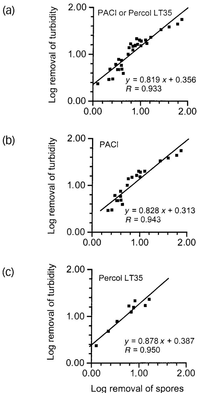
**Figure 1** | Relationship between the removal of aerobic spores and the removal of turbidity: (a) data from all trials, (b) data from trials using PACI only, (c) data from trials using Percol LT35 only.
