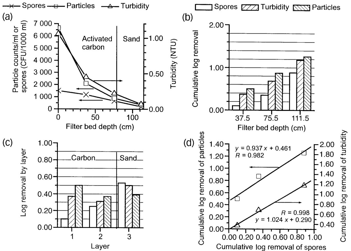
**Figure 4** | Monitoring the quality of the water as a function of depth in the filter medium, after 40 h 19 min of filtration, cycle No 580, Percol LT 35, 0.12 mg/l, 96/12/02: (a) variation of the total particle count (2–150 μm), turbidity and aerobic spores, (b) cumulative removal, (c) removal by the layers of filter medium (d) relationship between the removal of aerobic spores and the removal of total particle count or turbidity.
