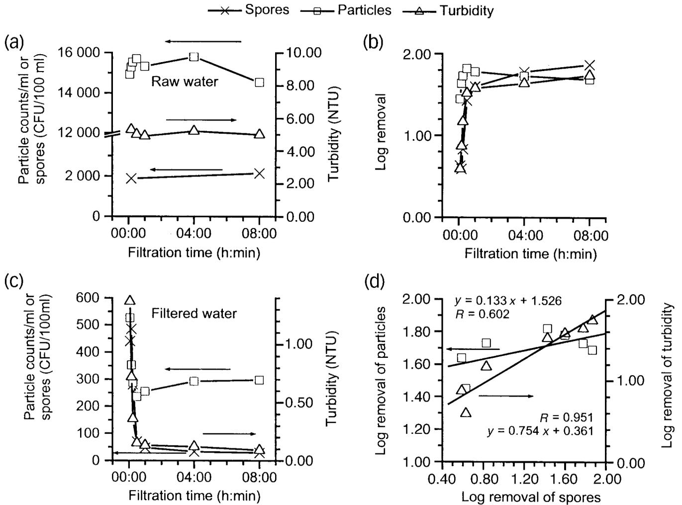
**Figure 6** | Monitoring the evolution of total particle count (2–150 μm), aerobic spores and turbidity, cycle No 367, PACI 17.5 mg/l, 96/04/30: (a) raw water, (b) log removal, (c) filtered water, (d) relationship between the removal of aerobic spores and the removal of total particle count or turbidity.
