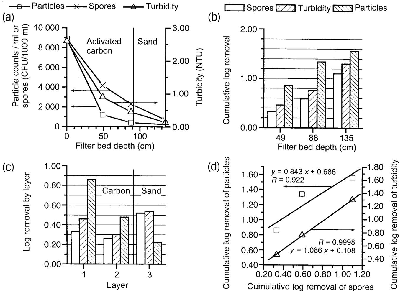
**Figure 3** | Monitoring the quality of the water as a function of depth in the filter medium, after 2 h of filtration, cycle No 358, PACl 10.0 mg/l, 96/04/23: (a) variation of the total particle count (2–150 μm), turbidity and aerobic spores, (b) cumulative removal, (c) removal by the layers of filter medium (d) relationship between the removal of aerobic spores and the removal of total particle count or turbidity.
