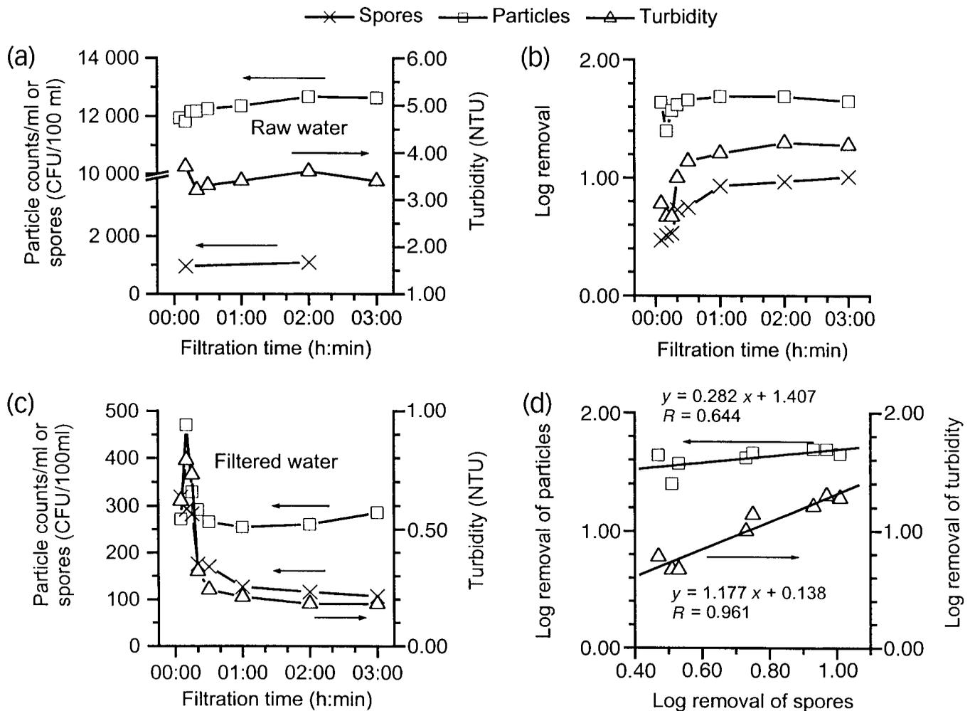
**Figure 5** | Monitoring the evolution of total particle count (2–150 µm), aerobic spores and turbidity during the first 3 h of filtration, cycle No 361, PACl 10.1 mg/l, 96/04/25: (a) raw water, (b) log removal, (c) filtered water, (d) relationship between the removal of aerobic spores and the removal of total particle count or turbidity.
