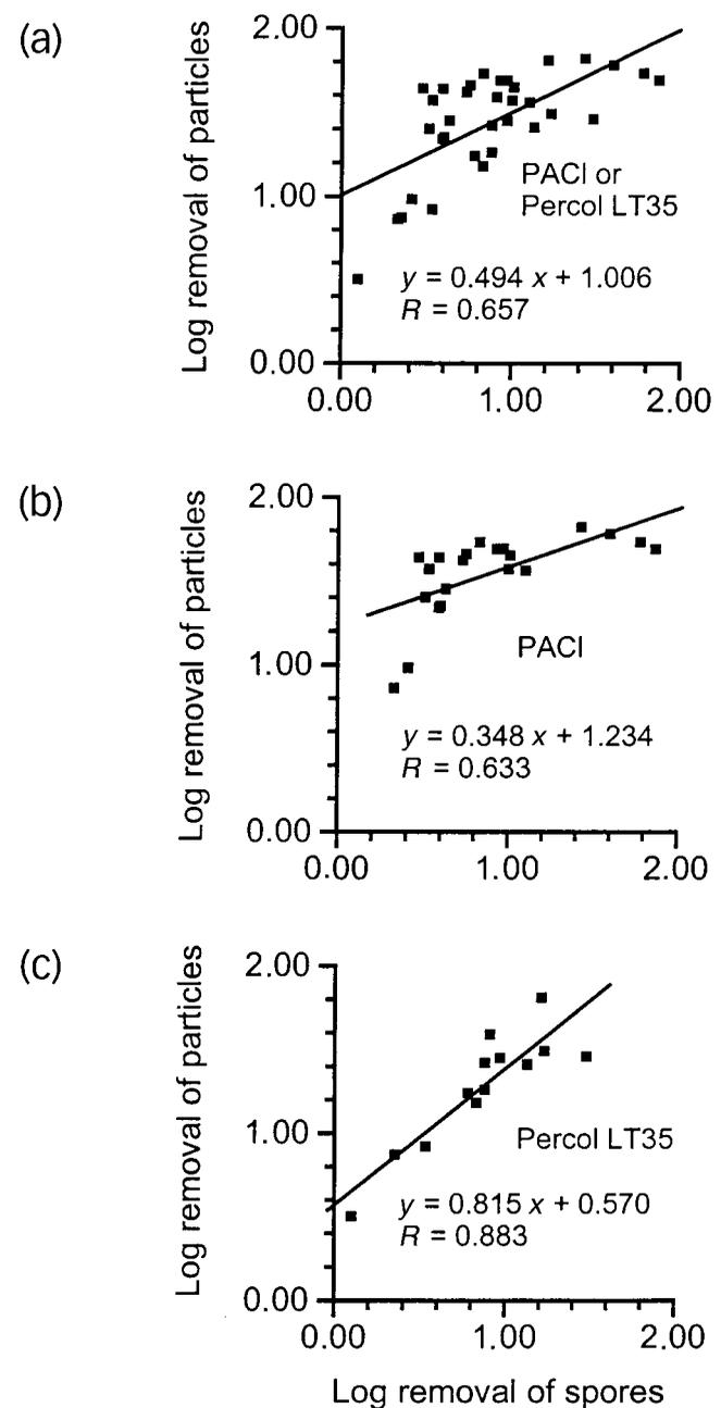
**Figure 2** | Relationship between the removal of aerobic spores and the removal of total particle count (2–150  $\mu\text{m}$ ): (a) data from all trials, (b) data from trials using PACI only, (c) data from trials using Percol LT35 only.
