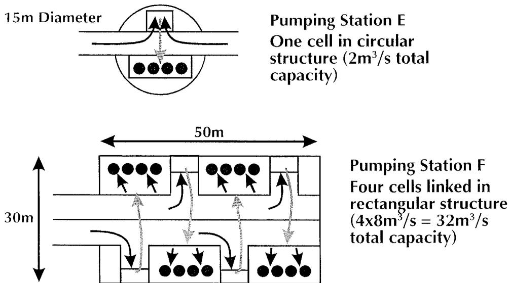
**Figure 3** | Stations E and F sumps compared.
