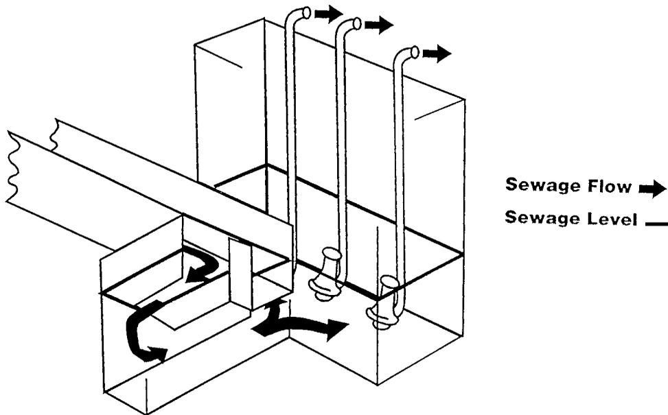
Figure 5 | The folded-over Sump Wells of Stations E and F.
