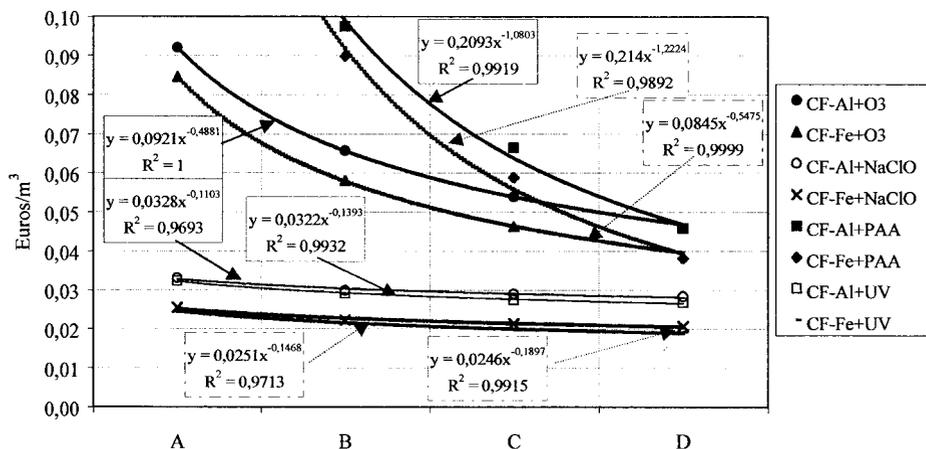
**Figure 6** Operation costs ( $\text{€}/\text{m}^3$ , amortisation not included) for different microbiological targets, in a 200,000 EI polishing plant (contact filtration + disinfection) using different chemicals and disinfectants (A = 2.2 T. Coli 100  $\text{ml}^{-1}$ ; B = 23 T. Coli 100  $\text{ml}^{-1}$ ; C = 100 T. Coli 100  $\text{ml}^{-1}$ ; D = 1,000 T. Coli 100  $\text{ml}^{-1}$ )
