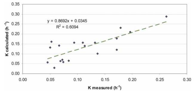
**Figure 3** | Relationship between the kinetic coefficients ( $K_{\text{cal}}$ ) and ( $K_{\text{meas}}$ ) for enterococci.
