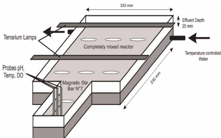
Figure 1 | Layout and photograph of laboratory pilot plant reactor.
