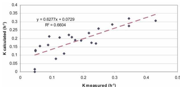
**Figure 2** | Relationship between the kinetic coefficients ( $K_{\text{cal}}$ ) and ( $K_{\text{meas}}$ ) for *E. coli*.
