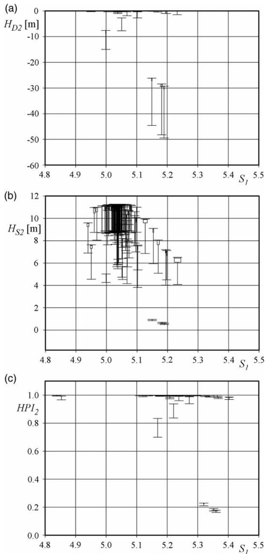
**Figure 8** | Network of Villaricca. Box plots of the distribution of hydraulic performance indices of all the network configurations with two link failures deriving from a *mother* network configuration with one link failure vs. entropy of the *mother* network: (a) mean hydraulic head deficit; (b) mean hydraulic head surplus; (c) hydraulic performance index.
