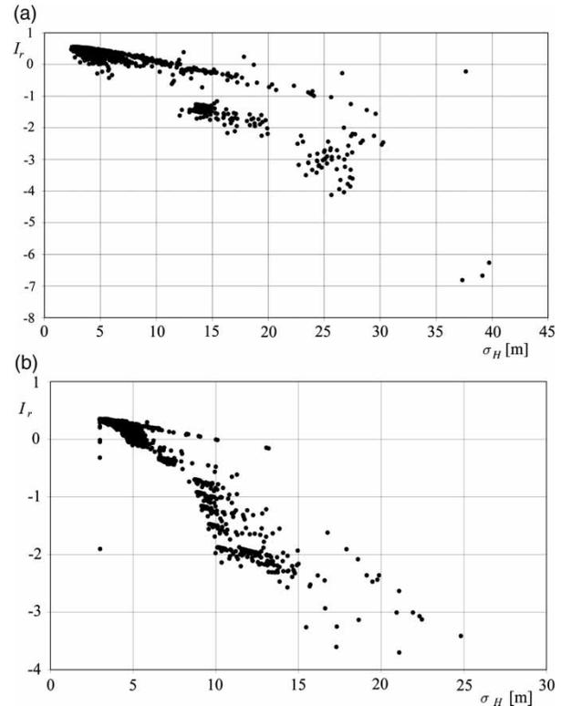
**Figure 5** | Scatter plots of resilience vs. standard deviation of hydraulic head at nodes: (a) network of Villaricca; (b) network of Parete.
