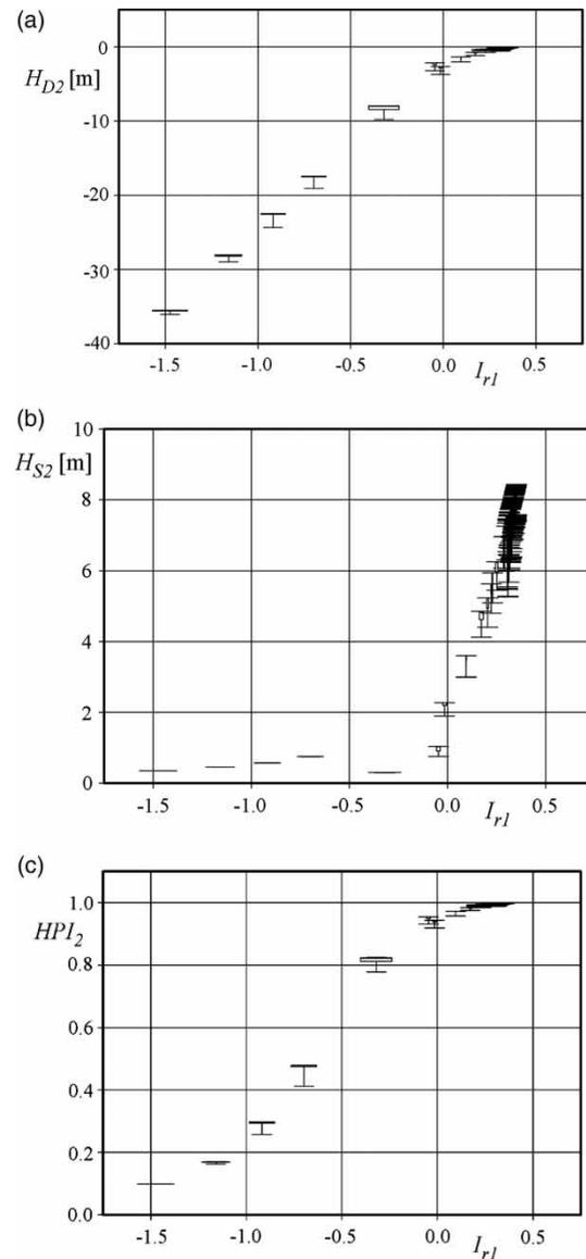
**Figure 9** | Network of Parete. Box plots of the distribution of hydraulic performance indices of all the network configurations with two link failures deriving from a *mother* network configuration with one link failure vs. resilience of the *mother* network: (a) mean hydraulic head deficit; (b) mean hydraulic head surplus; (c) hydraulic performance index.
