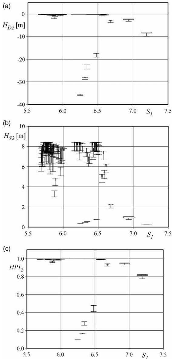
**Figure 10** | Network of Parete. Box plots of the distribution of hydraulic performance indices of all the network configurations with two link failures deriving from a *mother* network configuration with one link failure vs. entropy of the *mother* network: (a) mean hydraulic head deficit; (b) mean hydraulic head surplus; (c) hydraulic performance index.
