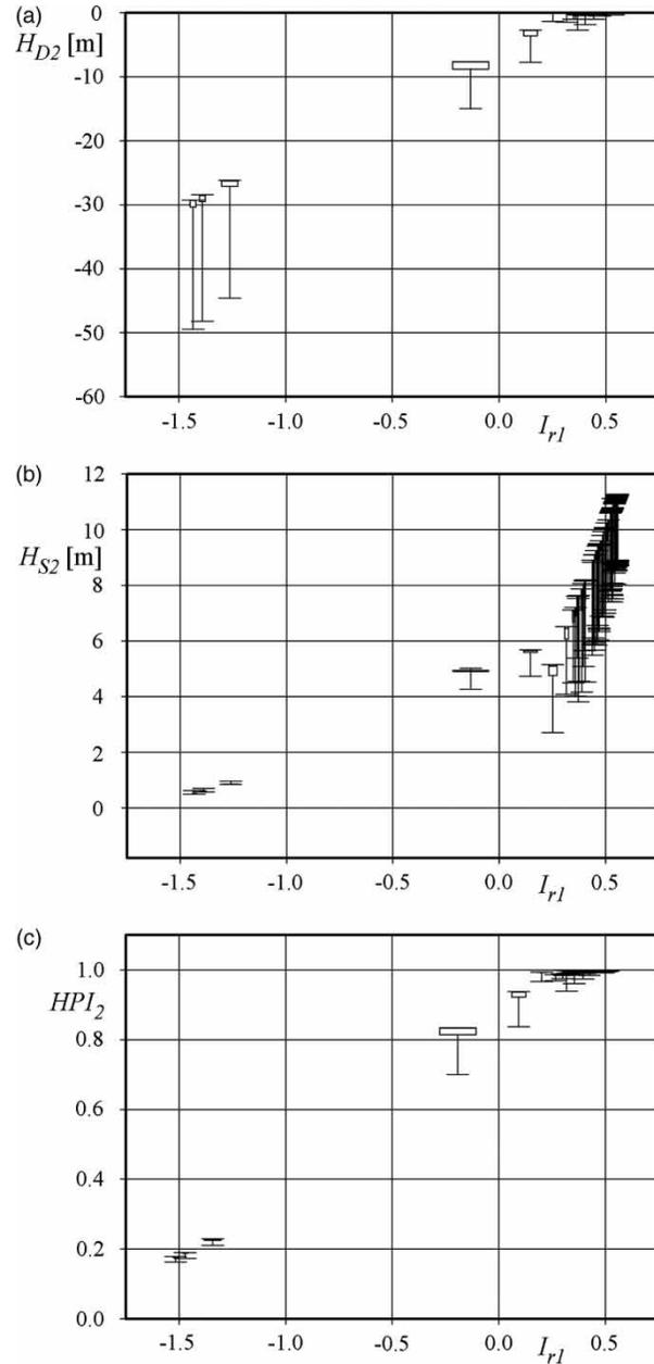
**Figure 7** | Network of Villaricca. Box plots of the distribution of hydraulic performance indices of all the network configurations with two link failures deriving from a *mother* network configuration with one link failure vs. resilience of the *mother* network: (a) mean hydraulic head deficit; (b) mean hydraulic head surplus; (c) hydraulic performance index.
