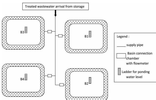
Figure 1 | Layout of the recharge basins in Souhil Wadi Facility.
