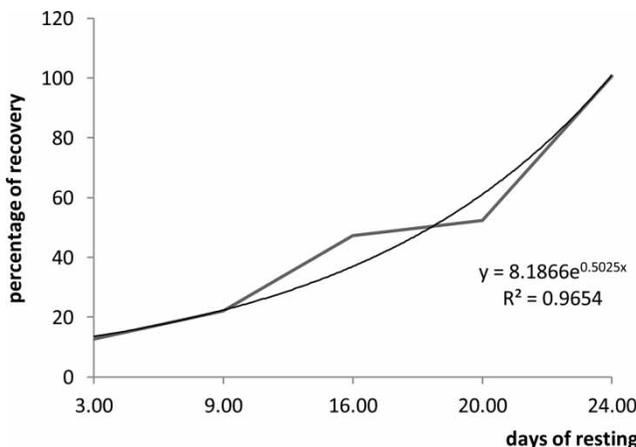
Figure 3 | Percentage of recovery of the clean water infiltration rate with resting days.
